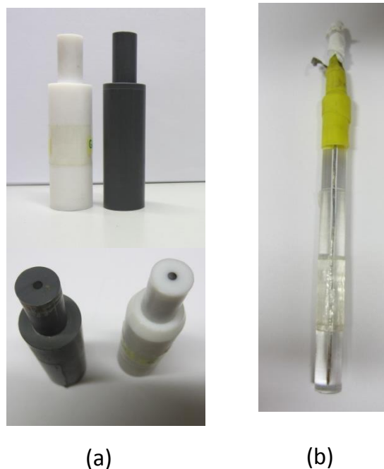
Figure 4.14. (a) Millimeter working electrode with PVC (blue) and Teflon (white) insulator; (b) micrometer working electrode.
