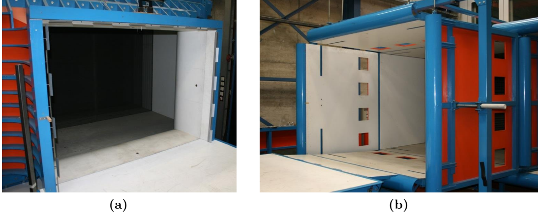
Figure 3.10: The 2m-wind tunnel of the Institute of Fluid Mechanics and Heat Transfer at Graz University of Technology. (a) Nozzle exit, (b) collector.
