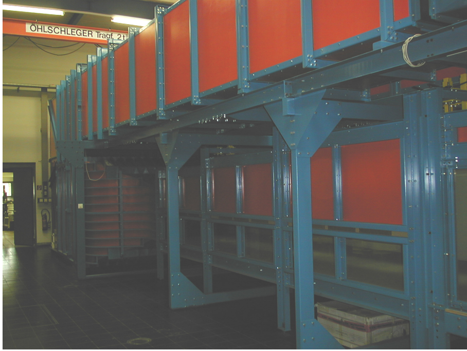
Figure 3.4: The boundary layer wind tunnel of the Institute of Fluid Mechanics and Heat Transfer at Graz University of Technology.
