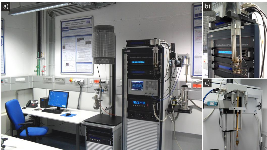
**Figure B.3:** a) Photograph of the impedance spectroscopy workstation Concept 80 (Novocontrol). Close-ups of the active ZGS sample cell (b) and the RF sample cell (c), respectively.
