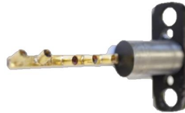
FIGURE 3: TOTAL PRESSURE RAKE PLANE C WITH TWO KIEL HOLES ALIGNED TO THE FLOW AT THE HUB OF THE INLET OF THE TMTF
