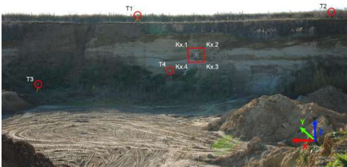
Figure 60: Overview of region of interest including control points and artificial rock with targets
