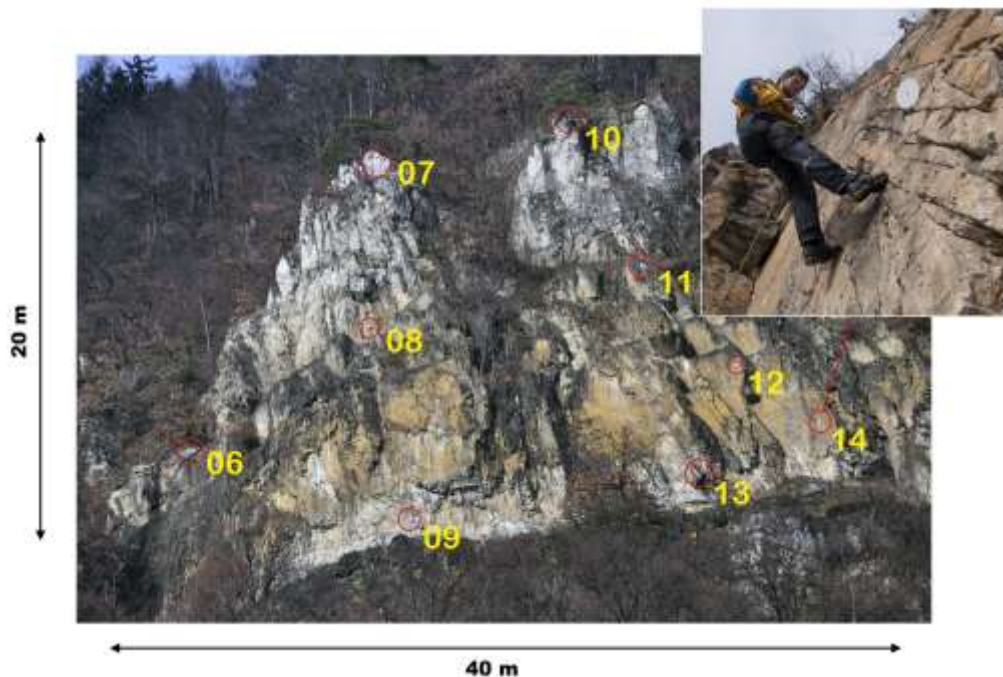
Figure 56: Measured Region of Interest, including numbered control points and close-up of mounting of target 14
