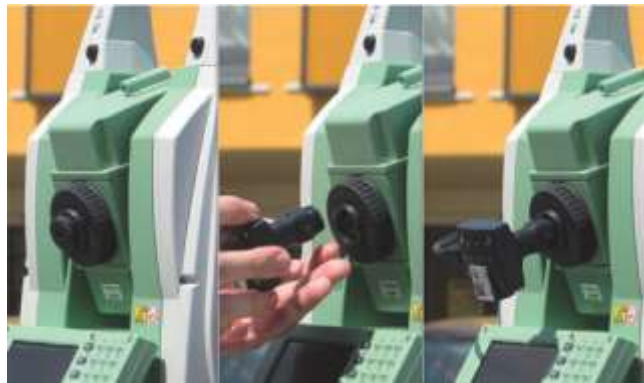
Figure 9: i3Mainz Digitalkameratachymeter mounting on a Leica TCRM 1103 (Hauth & Schlüter, 2010)
