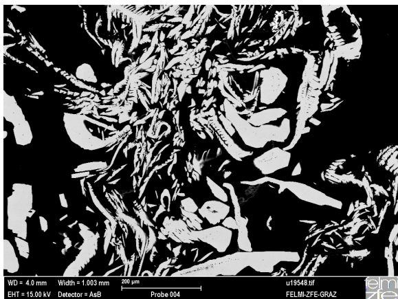
Figure 4.6: Morphology of the zinc deposits in charge.
