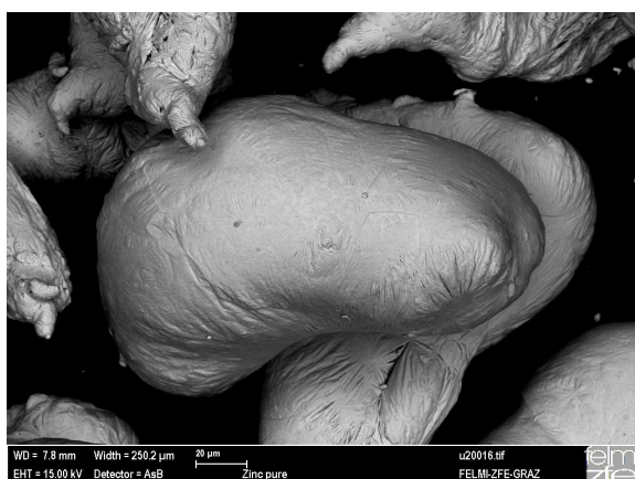
Figure 4.1: Zinc particle morphology.
