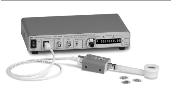
Figure 3.9: Quartz crystal microbalance apparatus.
