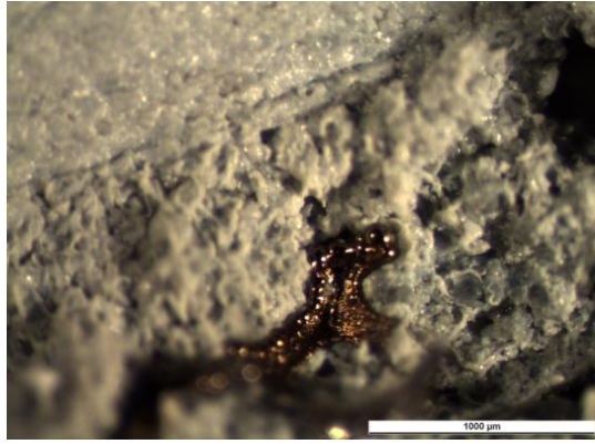
Figure 2.6: Area of a copper current collector of a rechargeable zinc electrode where the spontaneous zinc film deposit was stripped off upon repeated cycles. Source: Revolt Technology LLC.
