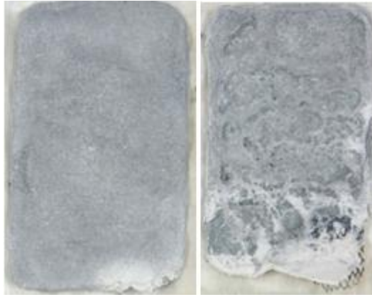
Figure 2.11: Morphology of prismatic zinc electrode after the 5 th cycle (left) and 80 th cycle (right) at 50% depth of discharge (source: Revolt Technology LLC.).
