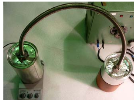
Figure C.2: Steam transferring from the boiling distilled water can go into the mineral oil can, while the mineral oil can is heated by the heating blanket about 40^{\circ}\text{C} - 60^{\circ}\text{C}
