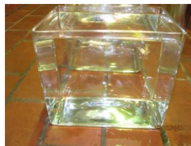
Figure C.3: Transferring the room temperature high water content mineral oil from the tin can to keep in the glass box before pouring into the test vessel for PDIV experiment
