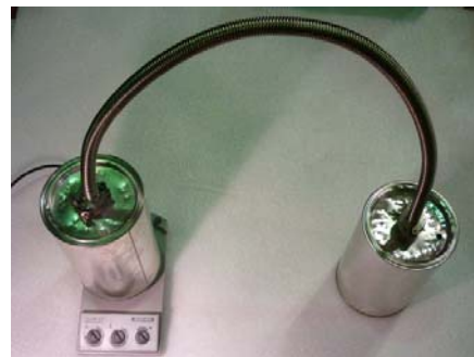
Figure C.1: Steam transferring from the boiling distilled water can go into the empty can
