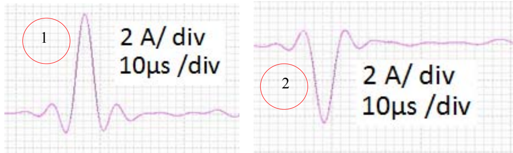
Figure 7.77: Arcing current patterns and signals tested by the rod- plane electrode arrangement, rod diameter of 1mm with gap distance of 0.3 mm at 11 kV
