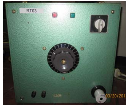
Figure D.2: Voltage controlled ac sources
