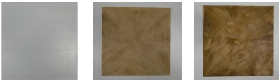
Figure 2-7 Reference plate PP (left), PP+2.5 wt% PI 2 (middle) and PP+5.0 wt% PI 2 (right)
