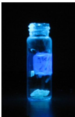
Figure 2-27 Polymer PI 4 under irradiation with UV light at a wavelength of 385 nm
