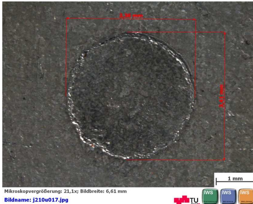
Figure 4.12: Stereoscope top down image of contact surface at the end of one period of current application
