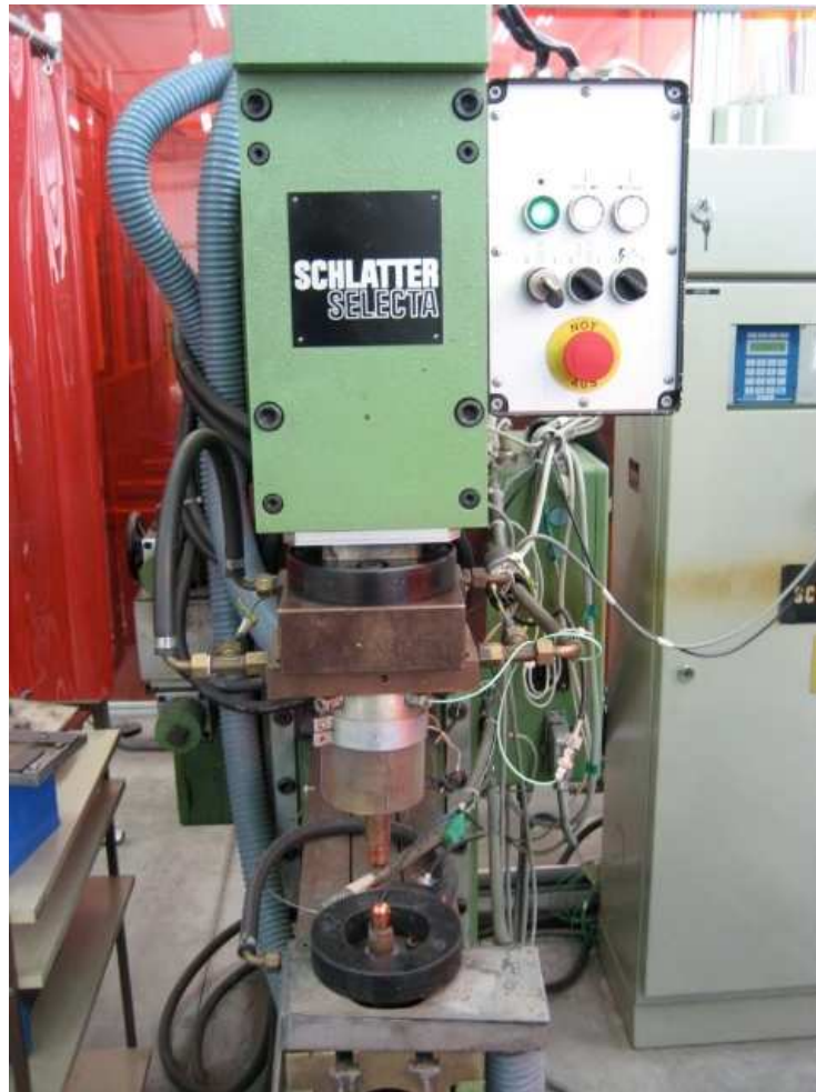
Figure 2.5: RSW machine, AC 170 kVA used in the welding experiments. All welding experiments were performed at voestalpine in Linz, Austria.
