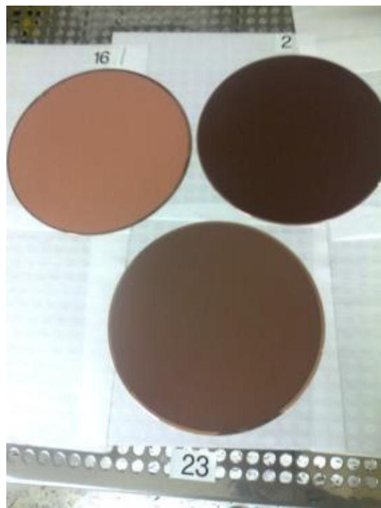
Picture 26: Comparison between an uncured wafer (2), a wafer processed at 400°C in forming (23) gas and a wafer processed at 400°C in formic acid (16)
