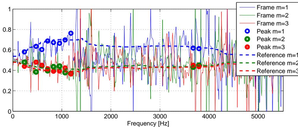
(c) *Feature curves*: At  $\varphi = 0^\circ$ , the first (blue) cardioid is stronger than the red and green one, which have the same level. This is reflected in the reference feature curves. The frame-features do only resemble the  $\varphi = 0^\circ$ -reference features at those frequencies where the source provides sufficient energy. Elsewhere, noise prevails and the  $\varphi = 0^\circ$  characteristic is not visible.
