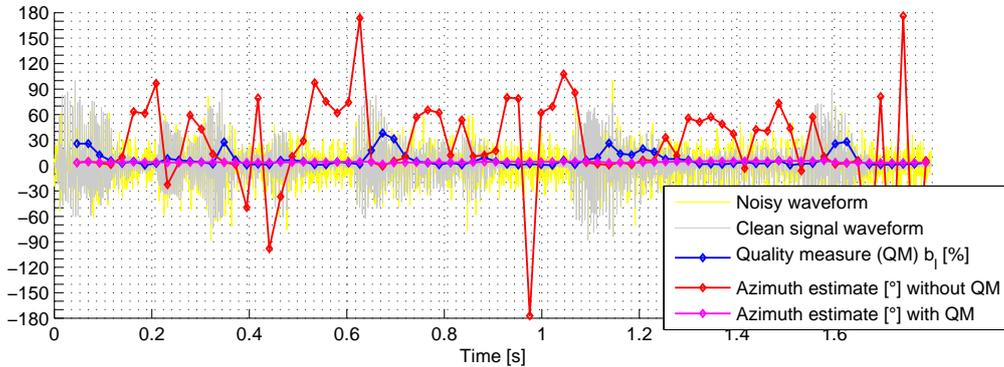
(b) Added omnidirectional pink noise (SNR=0dB) makes the unprocessed estimate (red) very erratic. The similarity variance quality measure (QM) is however still able to suppress all the 'bad' frames. The resulting magenta curve is again correct without outliers.
