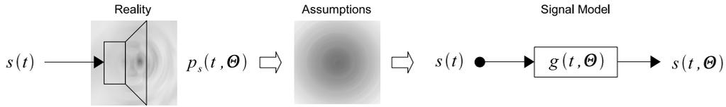
Figure 2.2: A sound source generates a sound field  $p_s(t, \Theta)$ . With the assumptions given in the text, a signal model can be introduced: A source signal  $s(t)$  drives an LTI-system  $g(t, \Theta)$  which models the dependence on the place of observation  $\Theta$ .
