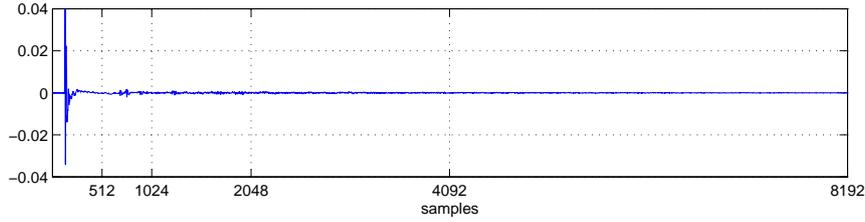
(a) Impulse Response of omnidirectional microphone  $h_0[n|\Theta = (\pi, 0, 1)$ , measured in Cube,  $f_s = 44100$  Hz. All information regarding the microphone is captured within the first 512 samples. Within 512 and 1024 samples, a prominent first reflection occurs. After 2048 samples the IR becomes diffuse, i.e. noisy.
