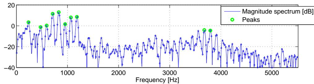
(b) *Magnitude spectrum* of the frame (a hanning-window was applied) depicted in Fig. 5.2a. The blue line is an interpolation obtained by zero-padding by a factor 4. The blue dots represent the  $N_x/2 + 1 = 266$  bins without zero-padding. The green circles indicate the result of the peak-picking routine ( $N_p = 10$ ).
