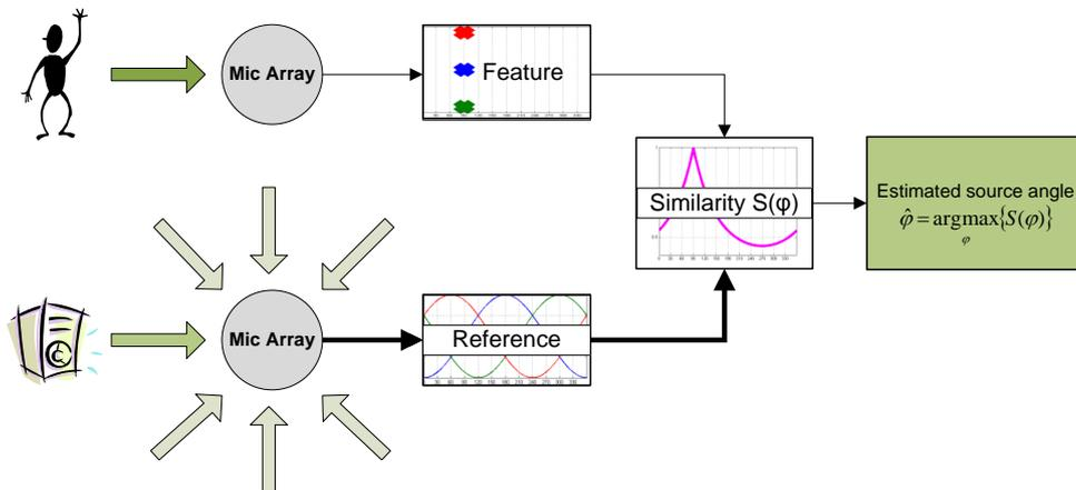
Figure 4.1: Supervised pattern classification principle: A reference database is obtained from measurements with a loudspeaker placed at different positions relative to the microphone array. An actual sound source, e.g. a human speaker, can be localized by computing a feature vector from the microphone signals and comparing it to a reference feature database. The database contains features belonging to different source positions.
