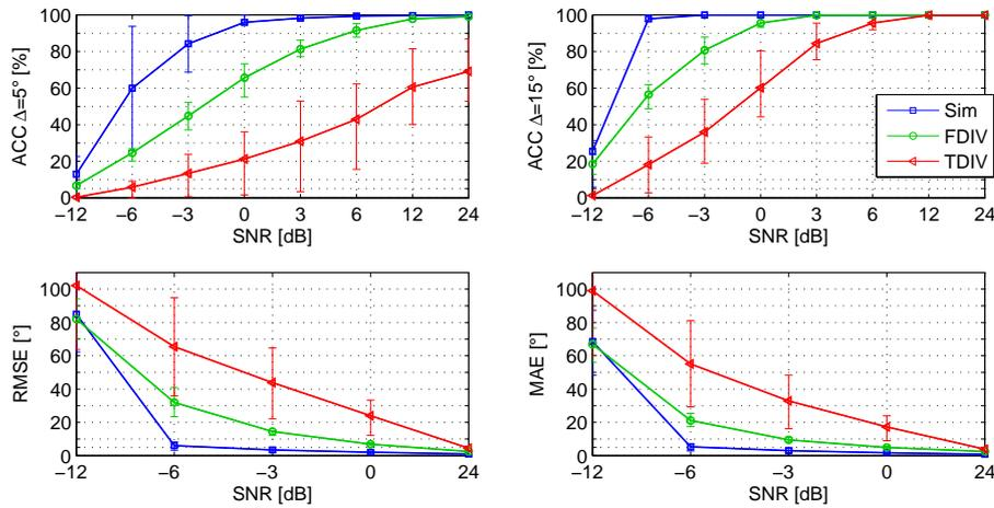
Figure 6.3: Different algorithm approaches: Mean over all source angles  $(-180, -170, \dots, 0)^\circ$  of  $ACC_{\Delta=5}$ ,  $ACC_{\Delta=15}$ ,  $RMSE$  and  $MAE$ , respectively. The errorbars indicate the first and the third quartile. This figure shows the same data as Fig. 6.4
