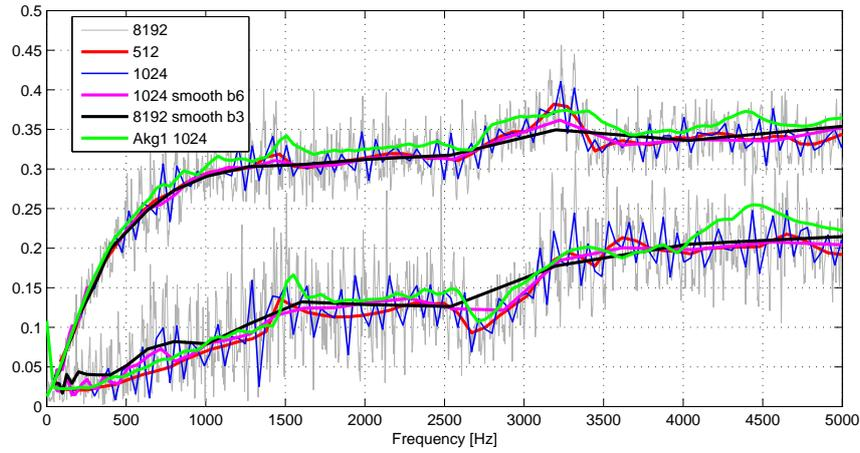
(b) Reference feature curves  $Y_m(f|\Theta = (\pi, 0, 1))$  for different window-lengths and smoothing coefficient  $b$ . The lower curves  $\mathcal{Y}_1$  belong to the first cardioid microphone  $m = 1$  which is off-axis, the upper curves show  $\mathcal{Y}_2 = |\frac{H_2}{H_0}|$ . A comparable curve measured in another room is shown (AKG1, hall-measurement).
