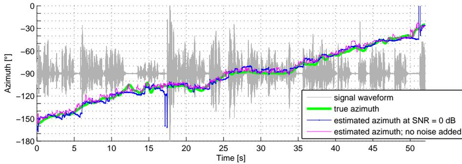
(b) Desk - Human speaker. A male person speaks while walking around the array. The elevation was between  $30^\circ < \vartheta_s < 40^\circ$ , the radius  $r_s \approx 1$  m.
