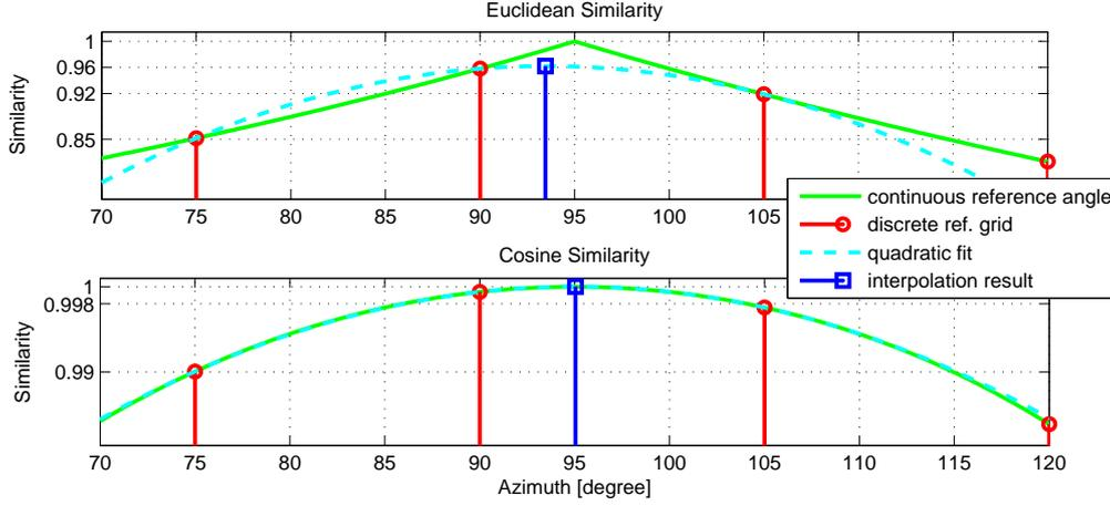
Figure 4.4: Parabolic Interpolation (PI): The true source angle is  $\varphi_s = 95^\circ$ . This angle is not contained in the discrete position grid  $\varphi_q = [75, 90, 105, \dots]^\circ$ . Without interpolation the estimated direction is hence  $\hat{\varphi}_s = \operatorname{argmax} \{S(\varphi_q)\} = 90^\circ$ . With PI however, an estimate in between  $90^\circ$  and  $105^\circ$  can be computed.
