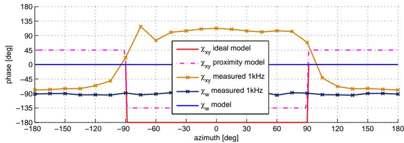
(d) Phase of the Eigenbeams: For perfect first order steering beams as in fig. 3.5a the on-axis half-plane must provide  $0^\circ$  phase-shift between  $\chi_w$  and the steered figure 8 pattern  $\chi_{xy}$ . Off-axis,  $180^\circ$  phase-shift are necessary for full cancellation. Only the ideal model fulfills these conditions perfectly.
