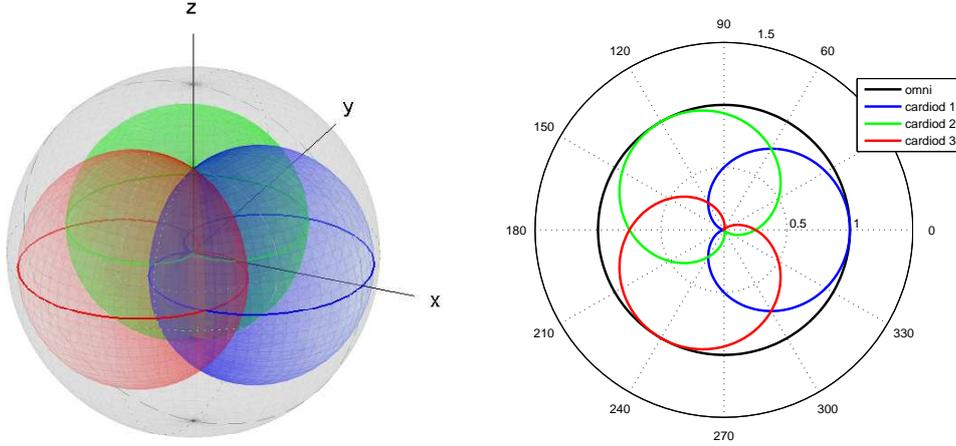
(a) Linear polar plot (3D): The sensitivity for sources from above, i.e.  $\vartheta = \pi$ , is the same for all microphones. (b) Linear polar plot (2D): The look directions of the cardioid microphones  $\varphi = (0^\circ, 120^\circ, 240^\circ)$  are clearly visible.
