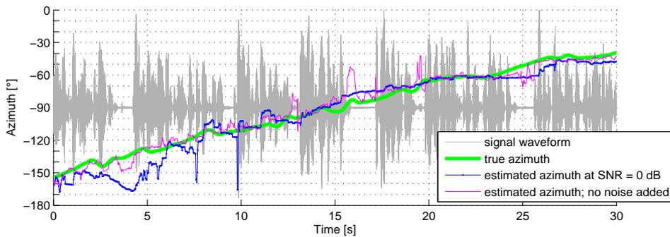
(d) Floor - Human speaker: Here the array was placed on the floor. Hence the elevation is higher ( $\vartheta_s \approx 60^\circ$ ). This is probably the reason, why the result is less accurate as in the case of the desk-setting.
