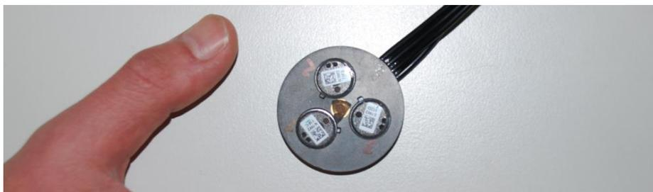
Figure 1.1: Coincident microphone array: prototype array
