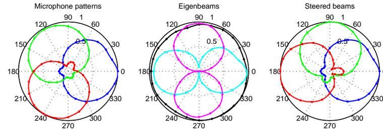
(c) Measured polar patterns at  $f = 1$  kHz and  $r = 1$  m: The shape of the steered beam patterns look slightly different for different steering angles.
