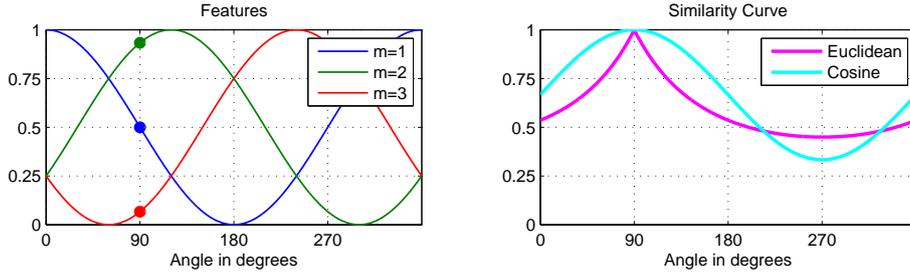
Figure 4.2: Similarity Principle: Assuming an ideal array (CMA1), the 3 dots in the left plot form the 3-element feature vector  $\mathbf{Y}$  produced by a source located at  $\varphi_s = 90^\circ$ . The curves represent the reference feature matrix  $\mathcal{Y}(\varphi_q)$ , i.e. a collection of feature vectors for different angles  $\varphi_q$ .
