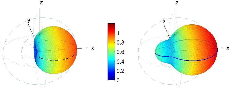
Figure 3.2: Proximity Effect: The picture on the left shows  $|H_{0.5}(f, \Theta)|$  for  $f = 10$  kHz and  $r = 0.5$  m, i.e.  $kr \approx 100$ . It virtually resembles the polar pattern of the ideal cardioid microphone without the proximity effect considered. Right:  $f = 100$  Hz, i.e.  $kr \approx 1$ . The boost compared to the left picture is clearly visible and especially pronounced off-axis, i.e. at  $180^\circ$ .
