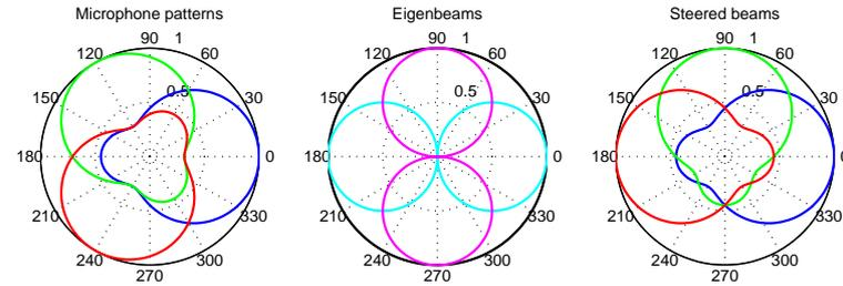
(b) Cardioid model incl. proximity effect for  $kr = 1$ . The eigenbeams  $|\chi|$  look just as in the case without proximity above. The steered patterns do however resemble the proximity cardioids and not a first order pattern. As explained in figure 3.5d this is because of the phase  $\angle\chi$ .
