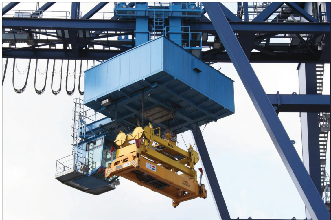
Figure 2-6 Crane Trolley and Spreader
