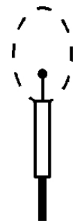
Figure 2.8: Preparation of the filaments, the dashed part is crushed in a vice.
