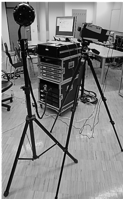
Figure 6.4: measurement setup in the IEM-library consisting of the spherical loudspeaker array, the LDV and the rack in the background containing the AD- and DA-converters, the amplifiers and the computer for PD
