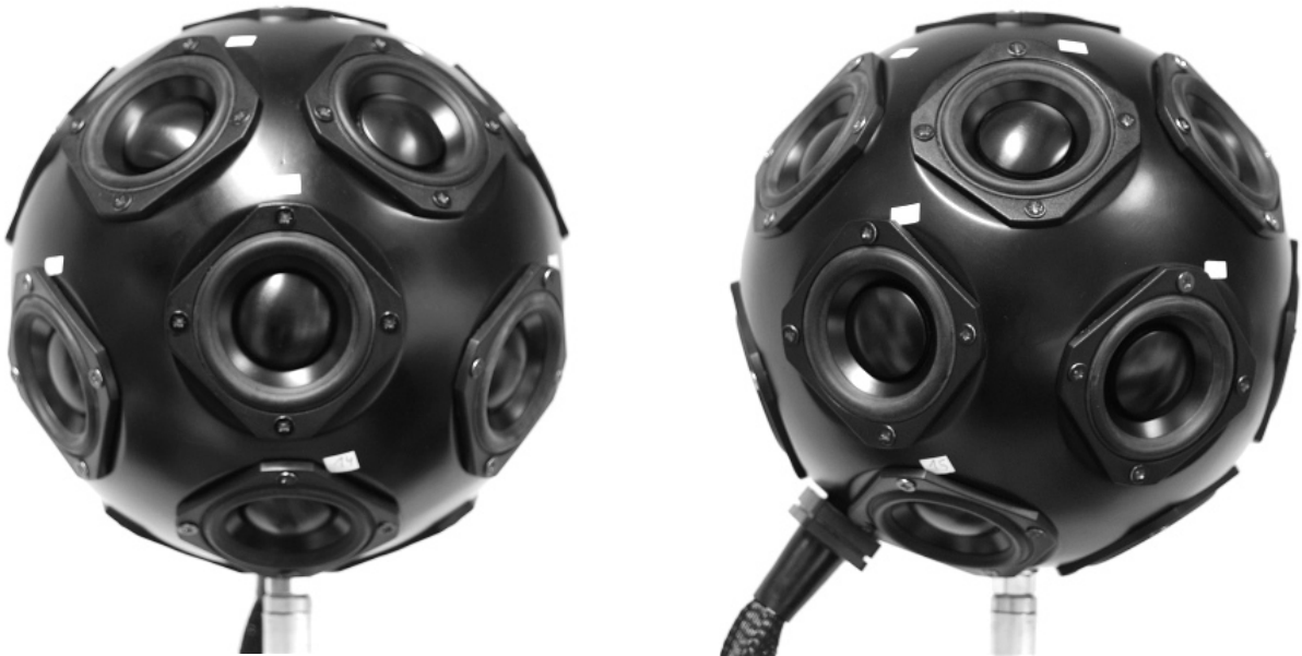
Figure 3.11: The final loudspeaker array: on the left seen frontally, on the right seen from the side
