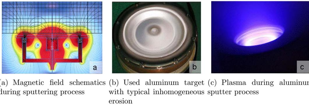
Figure 2.3: Magnetron sputtering process [Haas 06]
