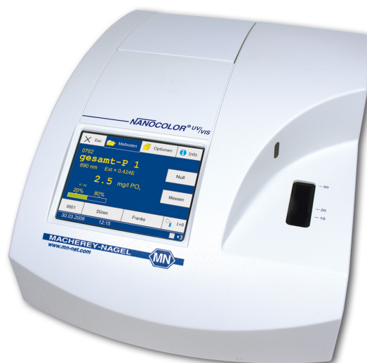
Abbildung 4.1: Spektralphotometer NANOCOLOR [Macherey-Nagel, 2010]
