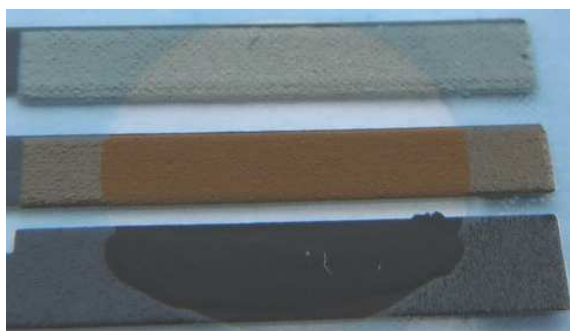
Figure 2.5: Electrochemical cell of a DuPont sensor with a bismuth film brushed on the carbon electrode.
