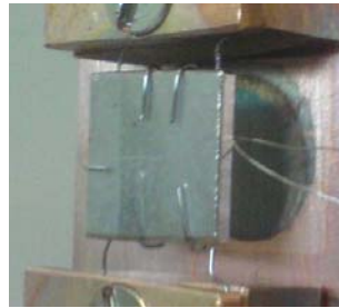
Figure A.1.: Mica mounted on the steel plate. The tantalum wires in the front fix the transparent mica sample on the plate, on these wires also 6P is deposited, hence in the TDS a so called 'tantalum' peak appears. The wires have nearly the same temperature as measured on the backside of the plate with the thermocouple on the right.
