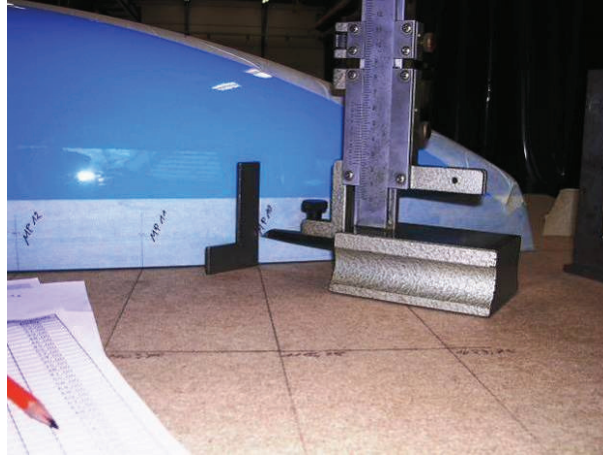
Figure 19: marking of the positions of the holes for the pressure measurements
