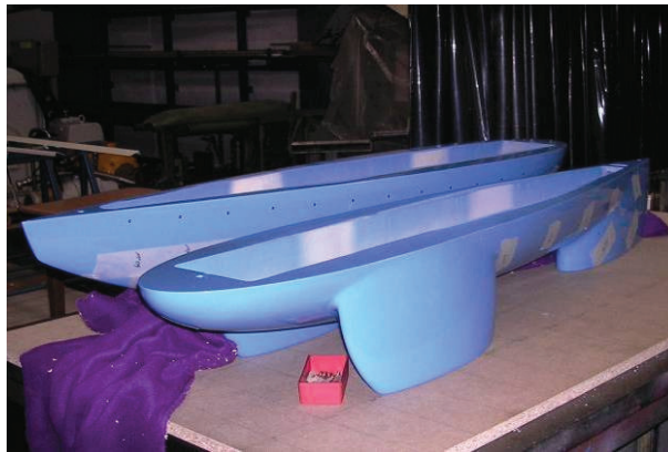
Figure 20: painted body with bore holes for the pressure measurements
