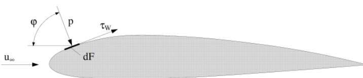
Figure 2: decomposition into pressure drag and viscous drag
