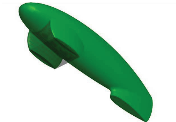
Figure 9: Venturi nozzle geometry between front wheel casings
