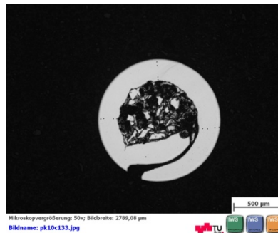
Figure 3-19: Wire cross section Masse 73
