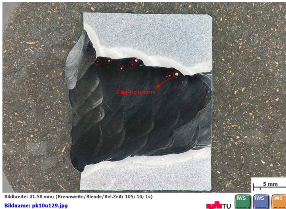
Figure 5-2: Alloy 625 multipass in horizontal vertical position (PC)
