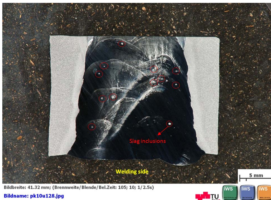
Figure 5-1: Alloy 625 multipass in overhead (PE) position
