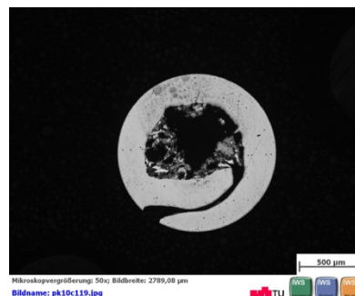
Figure 3-17: Wire cross-section Masse 68
