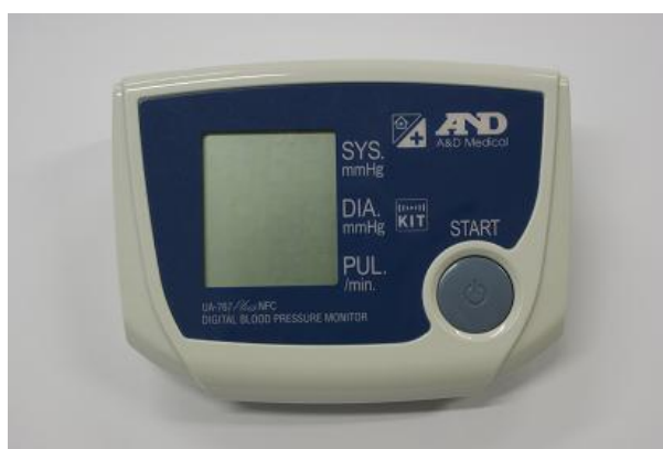
Figure 2.4: KIT enabled blood pressure monitor (UA-767 Plus NFC, A&D 10 ,Tokyo,Japan)
