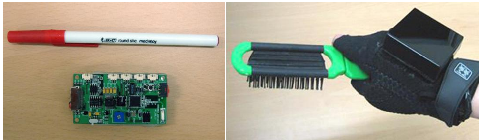
Figure 1.4: ZigBee based triaxial accelerometers (left) and RFID reader glove with tagged object (right)(Kim et al., 2007)
