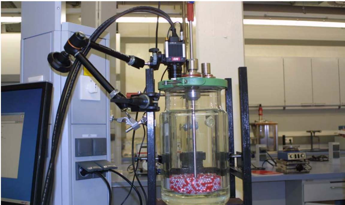
Figure 20: Photography of the vacuum dryer and the PIV camera
