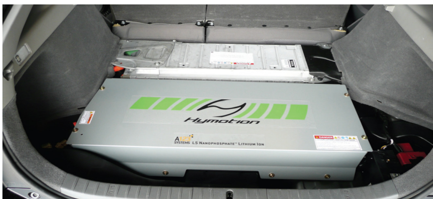
Figure 50: lithium ion battery in the Toyota Prius (Source: A123Systems)
