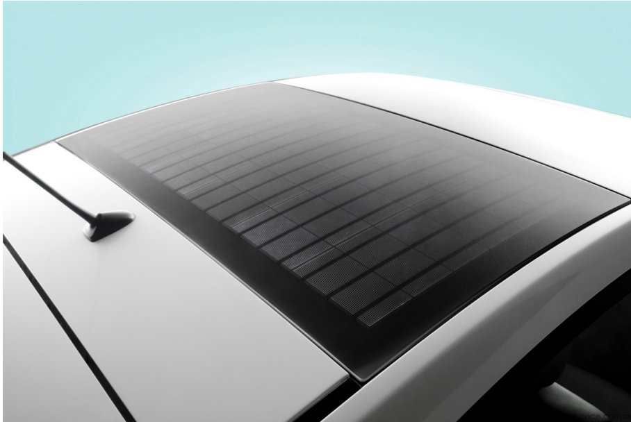
Figure 16: solar panel on Toyota Prius – figure (Source: Toyota)
