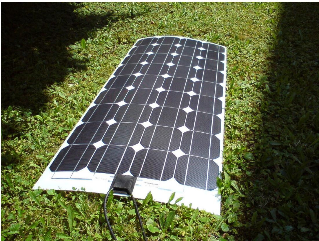
Figure 26: Encom HF80 solar panel in the sun at the time of measurement
