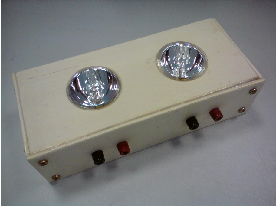
Figure 39: halogen lamp box with two lamps
