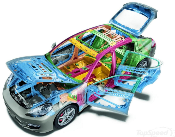
Figure 1.1: Porsche Panamera body structure, boron alloyed - red, polyphase - orange, micro alloyed - yellow, steel - green, aluminum - blue, magnesium torque [?]
