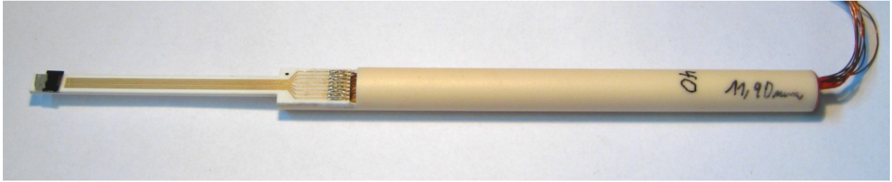
Figure 4.8: High temperature sensor mounting from AIT
