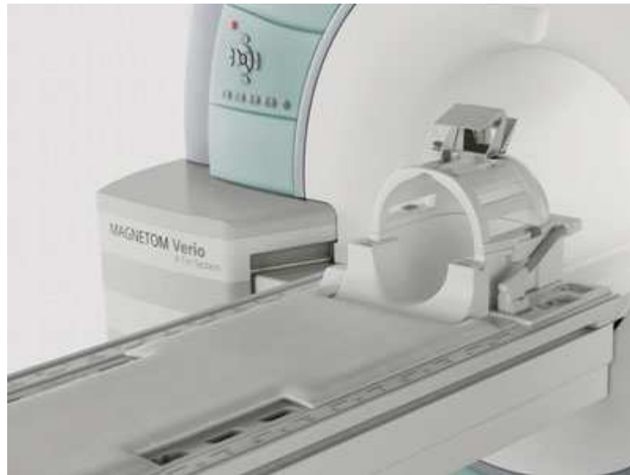
Figure 52: MRI RF coil and mirror attachment, used for motor imagery BCI (Siemens, 2002)
