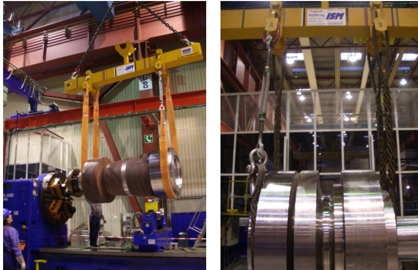
Fig. 3.8: Alignment of rotor modules
