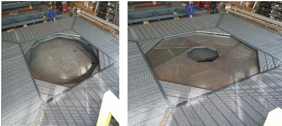
Fig. 4.6: Example of adjustable diaphragm [Polysoude 2010, p.71]
