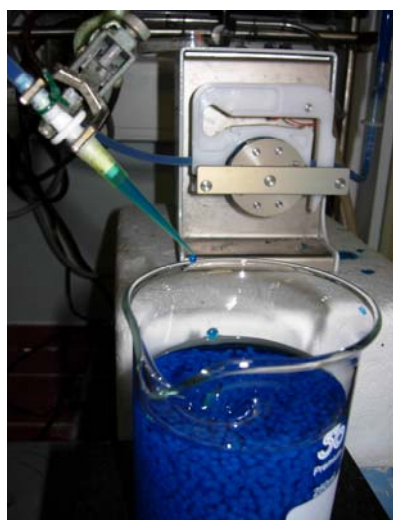
Picture 3: Fabrication of beads (picture kindly provided by Konstantin Schneider)
