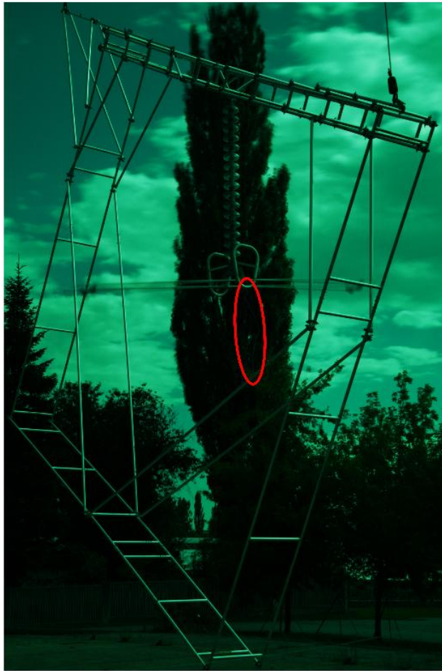
Figure 6.20: Flashover to the lower guy wire: SI – Test 1
