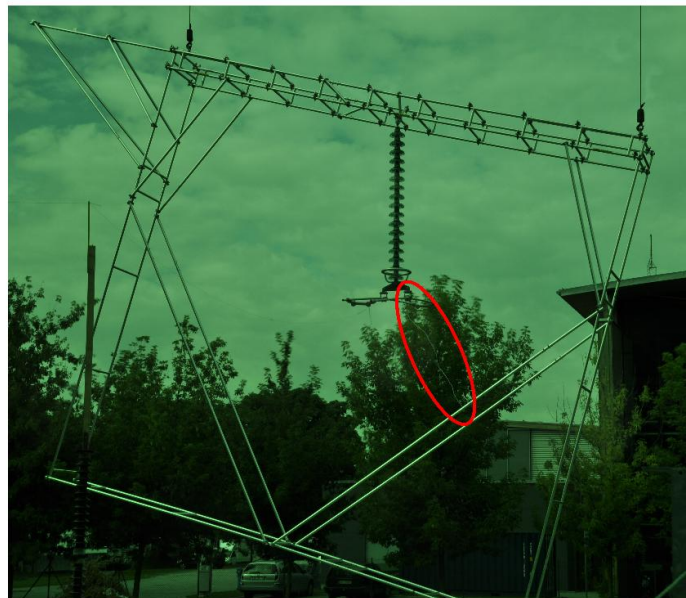
Figure 6.5: Flashover to the lower guy wire: LI – Test 2A
