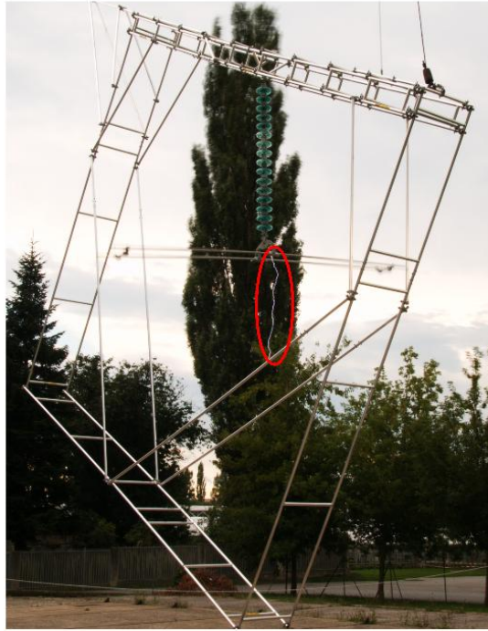
Figure 6.28: Flashover to the lower guy wire: SI – Test 1 (Bare insulator string)
