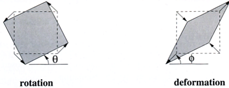
Figure 4.4: Distortions arising from the affine transformation. Rotation by R(\theta) and deformation R(-\phi)DR(\phi) . Note the scaling directions in the deformation are orthogonal. [30]
