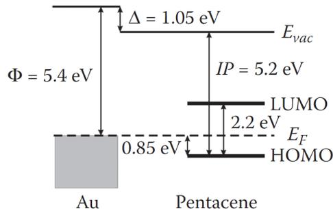
(b) Energy level alignment in the Au-pentacene junction, taken from Ref. [15]
