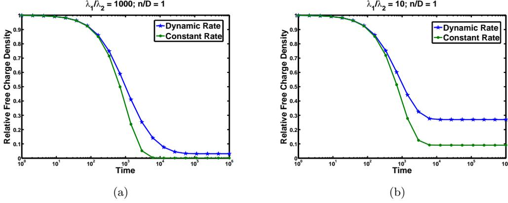
Figure 10.6.: Relative free charge density  $n_f/n$  with respect to the bias stress time for different  $\lambda_1/\lambda_2$  ratios.
