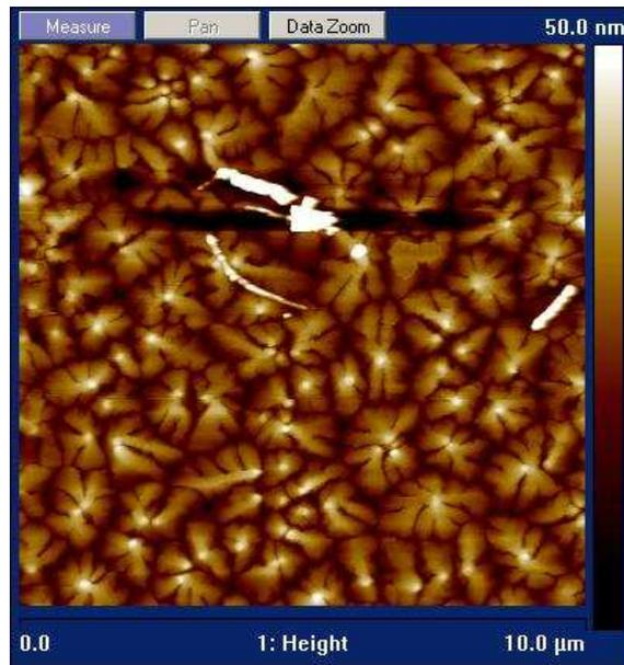
Figure 6.2.: AFM picture of the pentacene surface. Picture made by Anja Haase at NMP Weiz.
