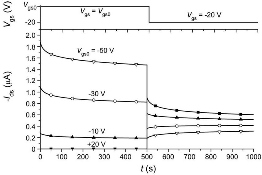
Figure 10.2.: Time dependent drain current under different gate bias stress. At  $t = 500s$  the gate bias was switched to  $V_G = -20V$ . It can be easily seen, that the equilibrium state is lying approximately at  $I_D = -0.5\mu A$ . Picture taken from Ref. [36]
