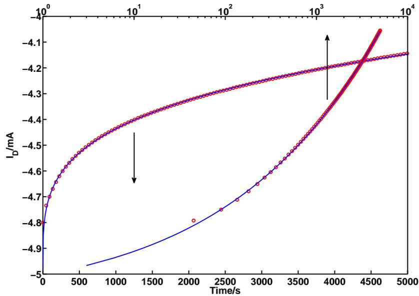
(b) Drain current over time on a linear and logarithmic scale. The solid line represents a fit to equation 11.1.
