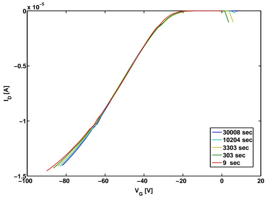
(a) Linear plot of drain current vs.  $(V_G - V_T)$  at different times. Shift of transfer line is not parallel.
