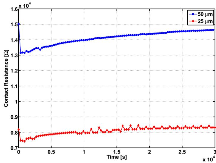
Figure 11.14.: Constant contact resistance obtained from the GDM a. CCR method for both channel lengths. Although the other parameters
