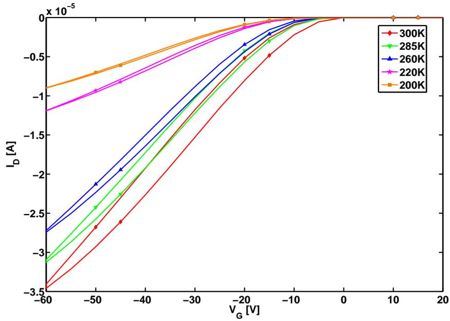
(a) Linear plot of transfer curves at different temperature.
