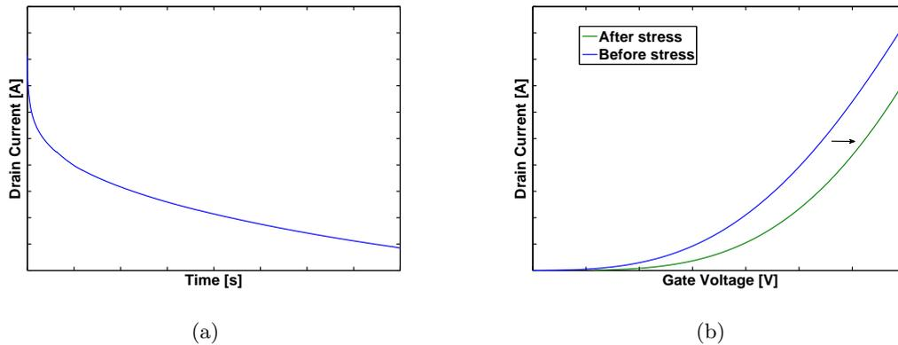
Figure 10.1.: Bias stress effect over 10 hours, measured on a top contact pentacene OFET: (a) Current degradation over time under inert conditions (b) the transfer curve shifts towards the applied voltage
