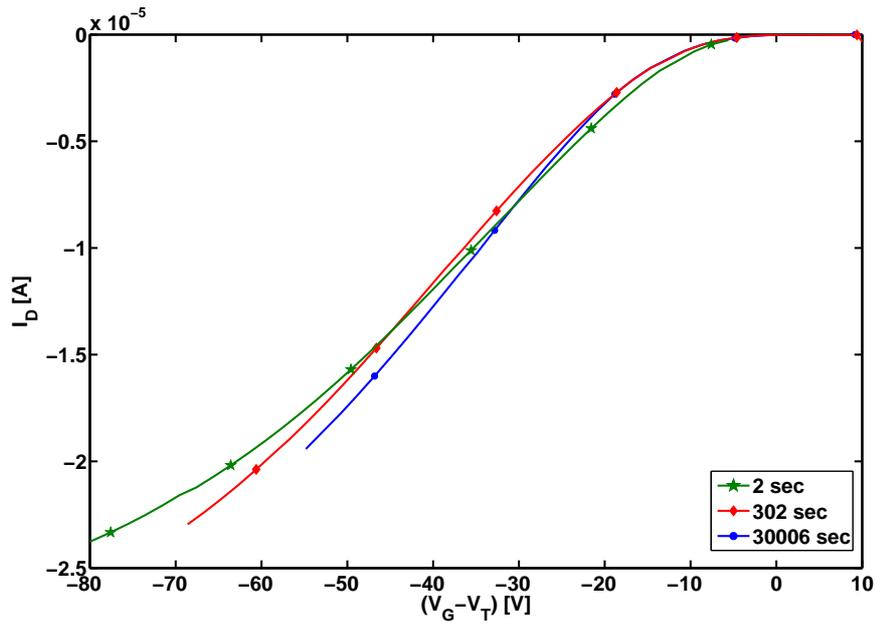
(a) Linear plot of drain current vs.  $(V_G - V_T)$  at different times. Shift of transfer line is not parallel.
