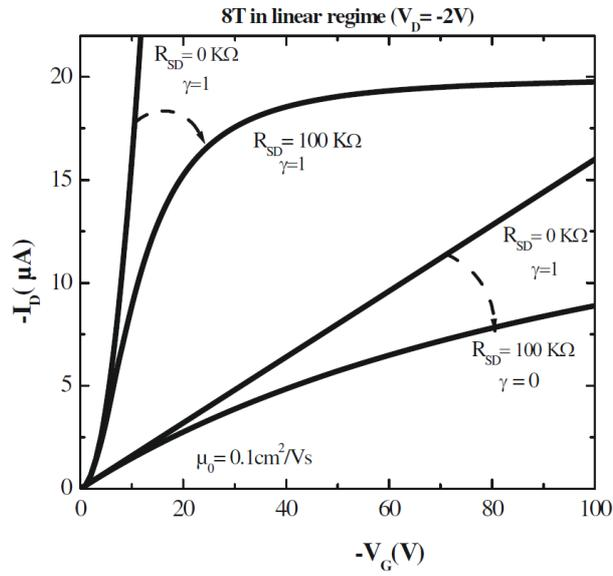
Figure 5.1.: Simulation of transfer characteristics in the linear regime according to equation 5.12; Picture take from Ref. [22]
