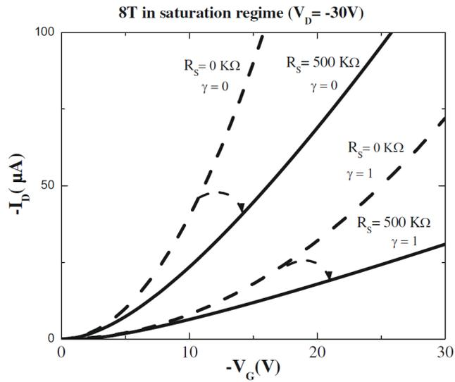
Figure 5.2.: Simulation of transfer characteristics in the saturation regime according equation 5.13; Picture take from Ref. [22]
