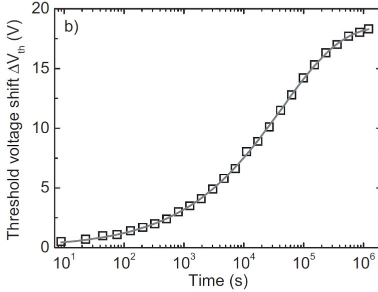
Figure 10.4.: Threshold voltage shift over time. The solid line represents a least-square fit to the stretched exponential model. Here, it is assumed that the threshold voltage shift after infinite time is equal to the applied voltage. Picture taken from Ref. [39].
