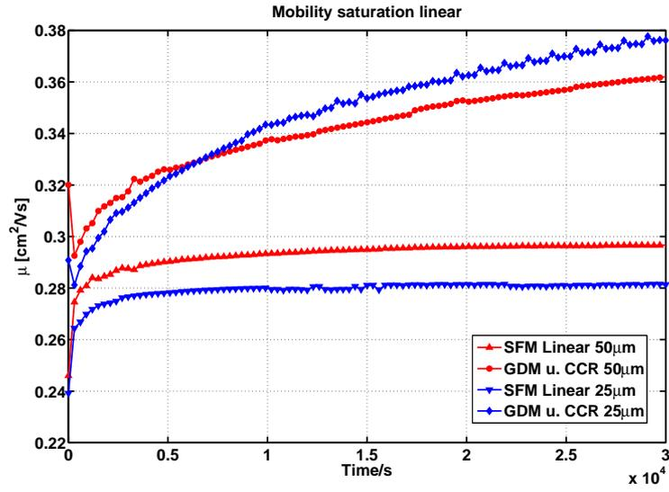
Figure 11.13.: Mobility vs Time; Comparison of the mobility values of GDM a. CCR and SFM linear method. Mobility values obtained from the GDM a. CCR method are estimated by  $\mu = \mu_0(-45V)^\gamma$ . Note that the mobility increases during the bias stress.
