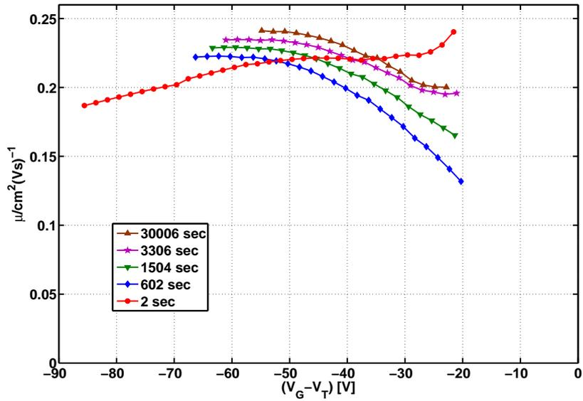
(a) Mobility vs. gate voltage minus threshold voltage at different times
