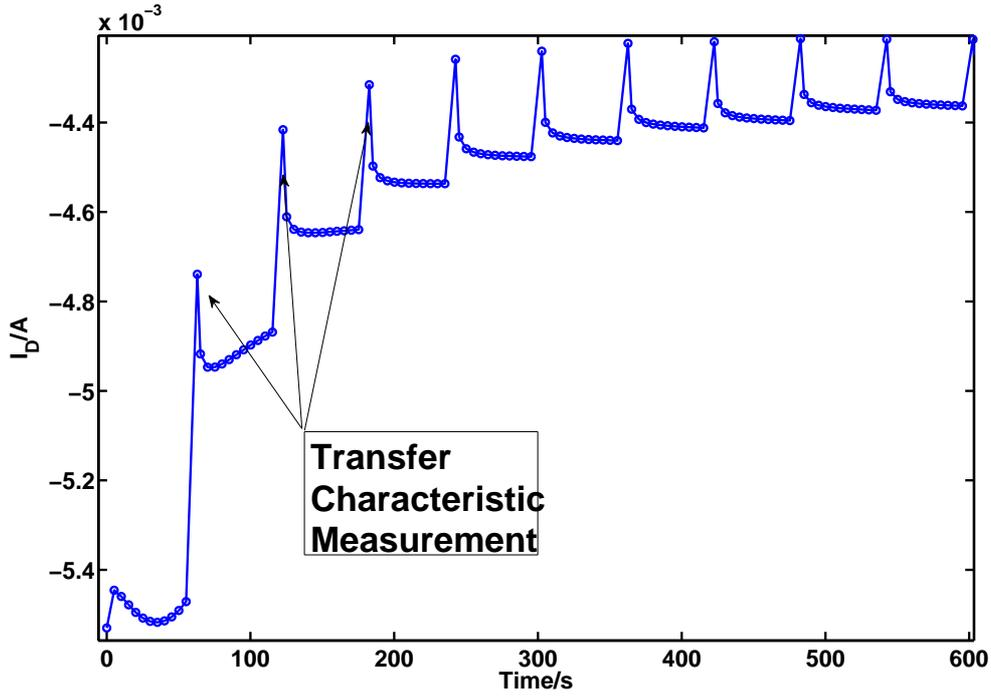
Figure 11.4.: Drain current dependence of time. Measuring transfer curves obviously affects the time dependence of the bias stress effect.
