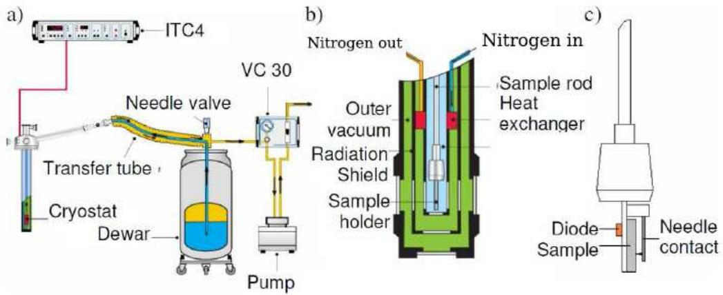
Figure 7.1.: (a) overview of the cryostatic setup. (b) Cross section of the sample space in the cryostat. (c) Sample holder. Picture taken from Ref. [48].
