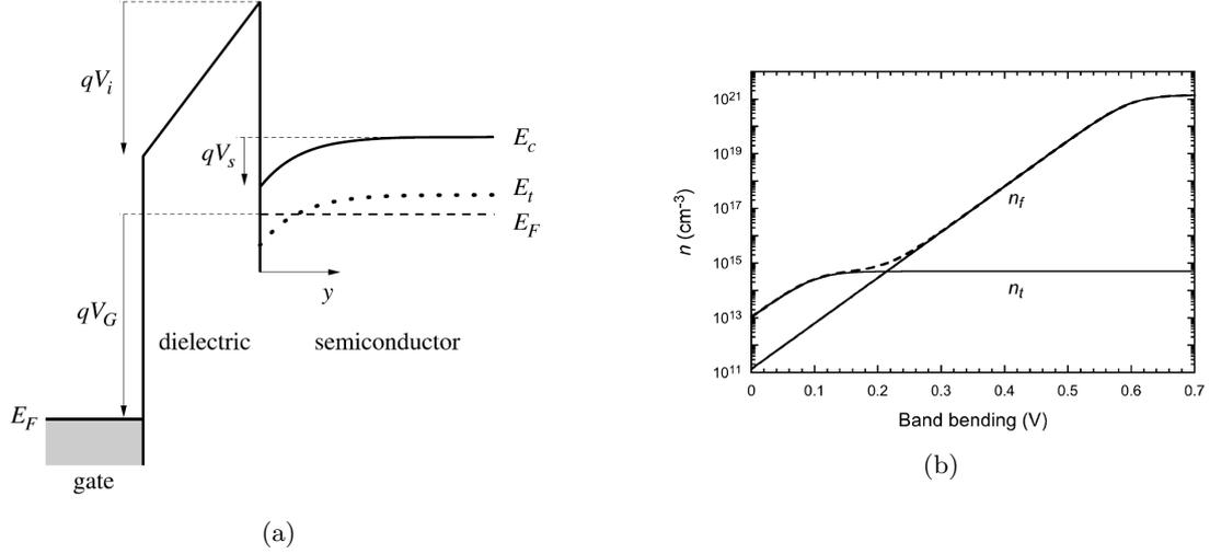
Figure 4.1.: (a) band diagram of a single shallow trap (b) free( $n_f$ ) and trapped( $n_t$ ) charge distribution as a function of the accumulation band bending; Pictures taken from Braga et al.[11]
