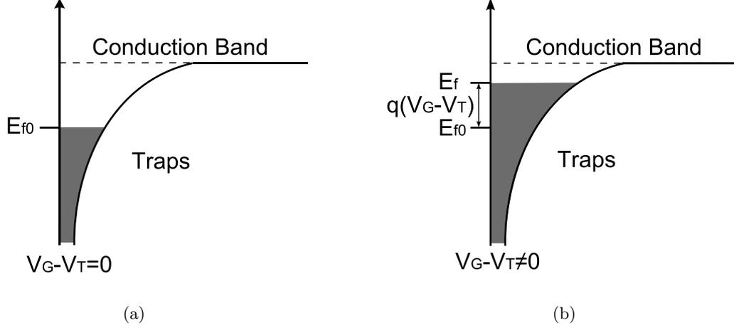
Figure 4.2.: (a) band diagram at zero bias (b) band diagram at nonzero bias
