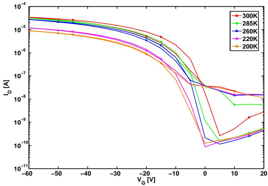
(b) Logarithmic plot of transfer curves at different temperature.
