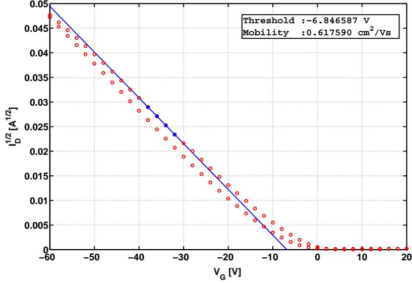
Figure 8.2.: Square root current as a function of the gate voltage. Transfer line record at  $V_D = -45V$ . Blue line represents the linear fit according to equation 8.2.
