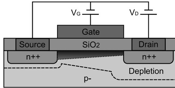
Figure 3.1.: Cross-section of an Metal-Oxide-Silicon-Field-Effect-Transistor
