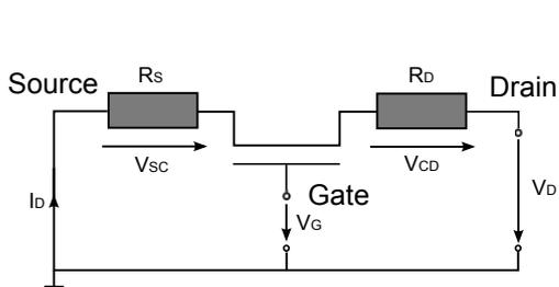
(a) Equivalent circuit diagram of an OTFT with contact resistance
