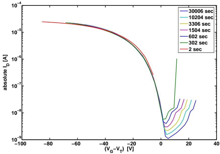
(b) logarithmic plot drain current vs.  $(V_G - V_T)$  at different times. Onset Voltages match each other.
