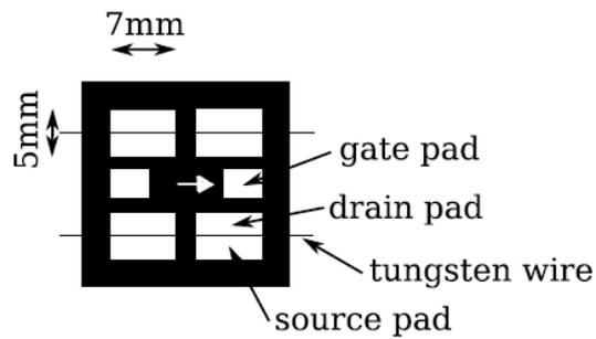
Figure 6.3.: Shadow mask through which gold contacts were evaporated on top of the semiconductor. Four devices with two common gate contacts were realized in this setup.
