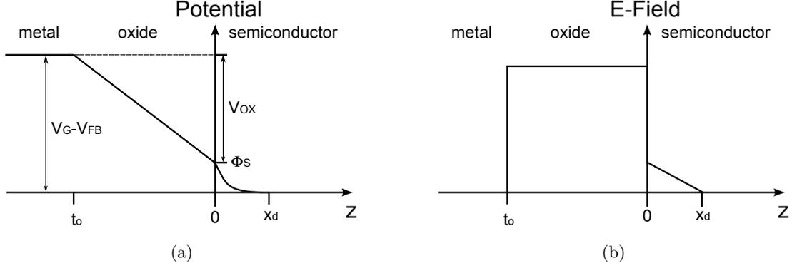
Figure 3.3.: Electrostatical analysis of a MOS structure: (a) the potential, (b) the electric field
