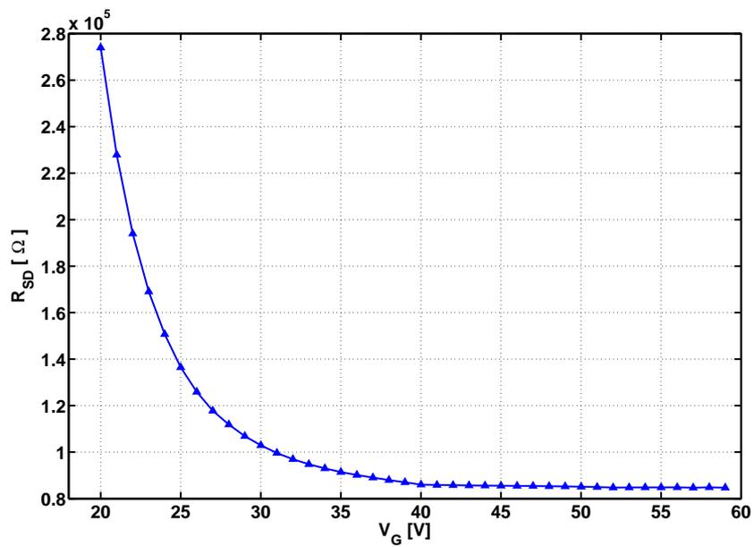
Figure 8.5.: Contact resistance versus gate voltage. Values obtained by the Natali method with equation 8.7. Transfer characteristic of a pentacene OTFT has been measured at  $V_D = -0.5V$ .
