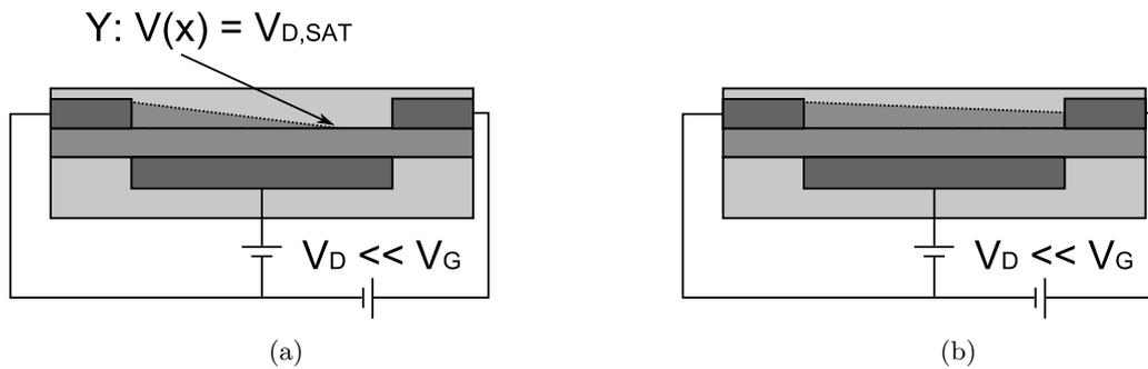
Figure 2.2.: (a) saturation regime (b) linear regime; the shaded areas in the channel indicates the charge carrier distribution
