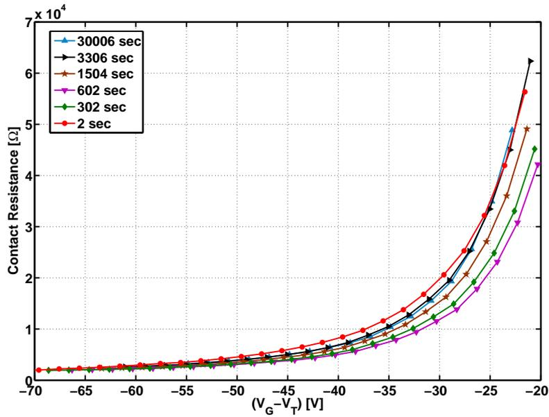
(b) Contact Resistance vs gate voltage for different progress times of the bias stress.
