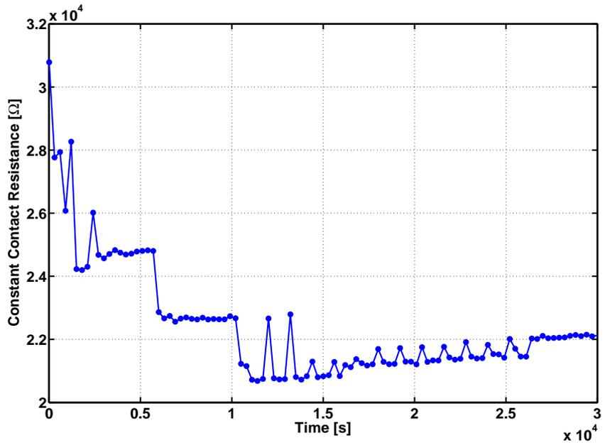
(b) Constant contacted resistance obtained from GDM a. CCR method.
