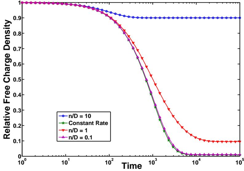
Figure 10.5.: Time dependence of the relative free charge density  $n_f/n$  for dynamic rate coefficients at different values of  $n/D$ , according equation 10.24, and for constant rate coefficients, according equation 10.16. The  $\lambda_1/\lambda_2$  ratio was set to 100.
