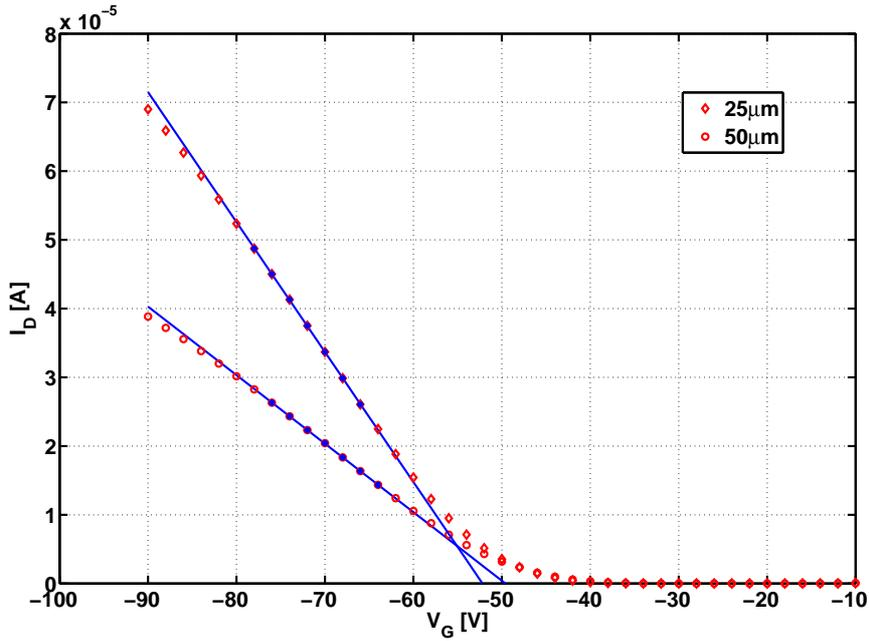
Figure 11.6.: Two fits with SFM linear method for two different channel lengths. Both transistors are fabricated on the same substrate and exhibit the same on-set voltage. However, the threshold voltages, which are extracted with SFM method linear, are not the same.
