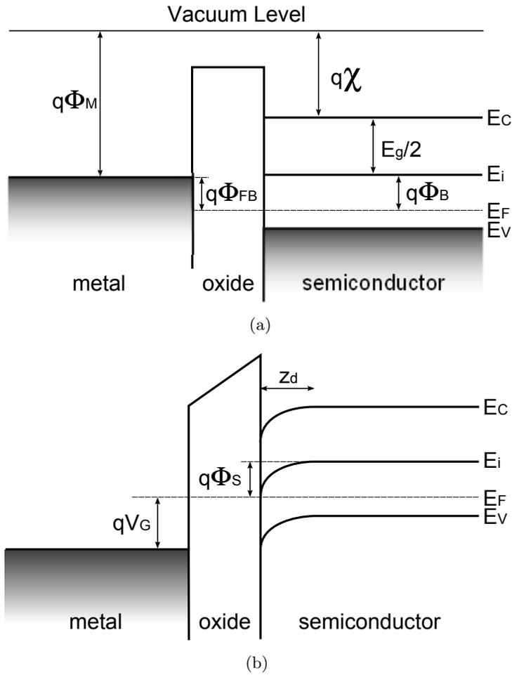
Figure 3.4.: Band diagrams of an MOS structure: (a) at flat band voltage and (b) at transition from depletion to weak inversion;  $E_i$  is the Fermi level of an undoped semiconductor. The difference of Fermi level  $E_F$  and  $E_i$  is proportional the bulk potential  $\Phi_B$ .  $\chi$  is the electron affinity in the semiconductor.  $E_g$  labels the energy gap between conduction band edge  $E_C$  and valence band edge  $E_V$ .
