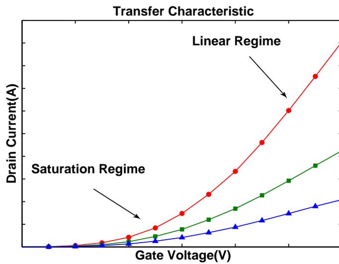
Figure 2.3.: Current-voltage characteristics of a pentacene OTFT :(a) Output characteristics; here one sweeps drain voltage at fixed values of gate voltage; (b) Transfer characteristics; here one sweeps gate voltage at fixed values of drain voltage
