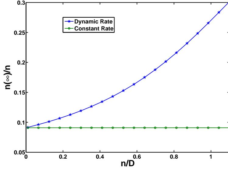
Figure 10.7.: Free charge density in the equilibrium state with respect to the trap site to induced charge ratio, according to equation 10.17 and equation 10.28.
