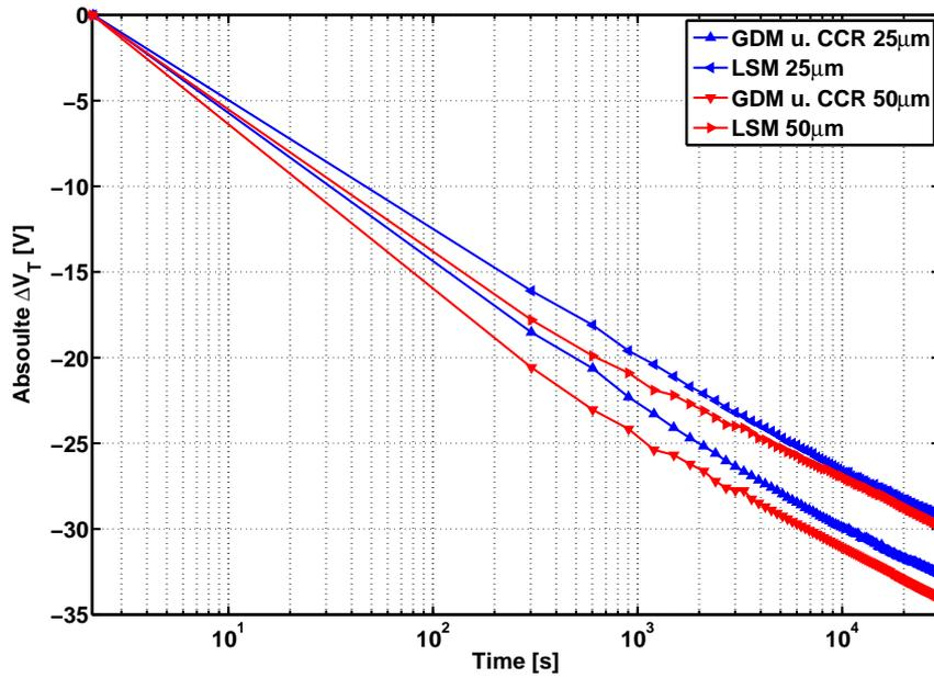
(b) Logarithmic plot of absolute threshold shift vs. Time.
