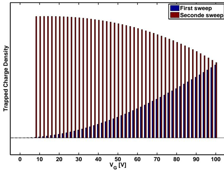
(b) Trapped charge density vs gate voltage.
