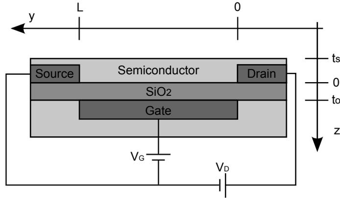
Figure 2.1.: Schematic structure of an field-effect transistor and applied voltages:
