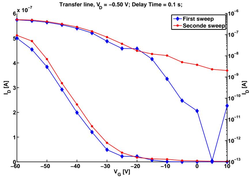
(a) Drain current vs gate voltage. Delay time between each measurement point was 0.1 seconds.
