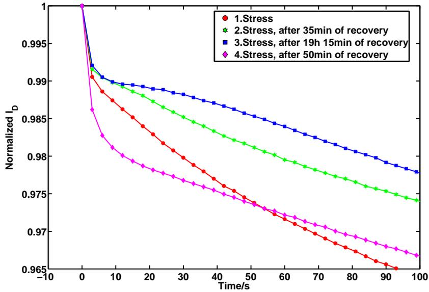
(a) Normalized drain current values within the first 100 seconds. At the beginning the drain current degradation is not exclusively dominated by the bias stress effect.
