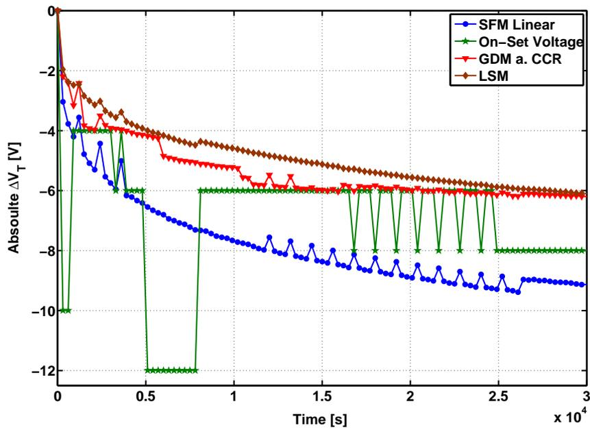
(b) Absolute threshold voltage shift  $\Delta V_T$  vs Time.
