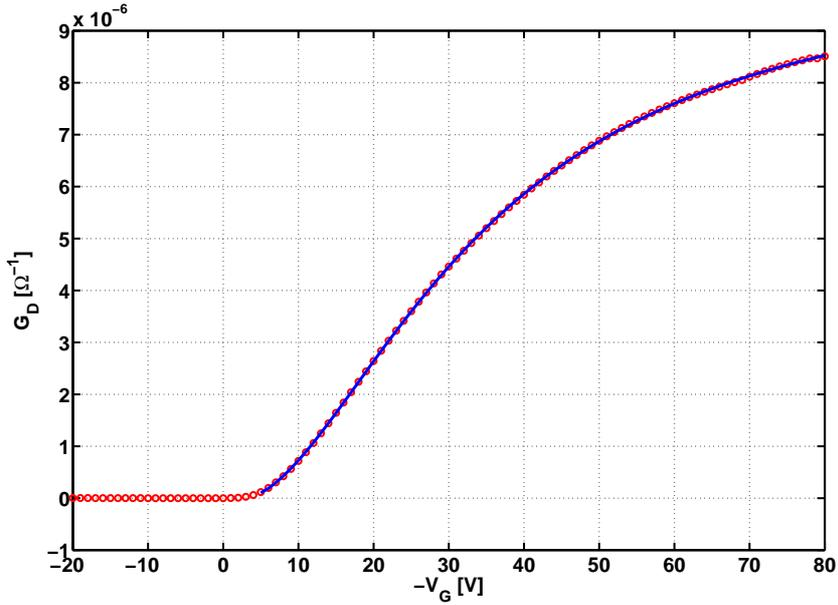
Figure 8.3.: Conductance versus absolute gate voltage. The solid line represents a least-square fit to equation 8.4.
