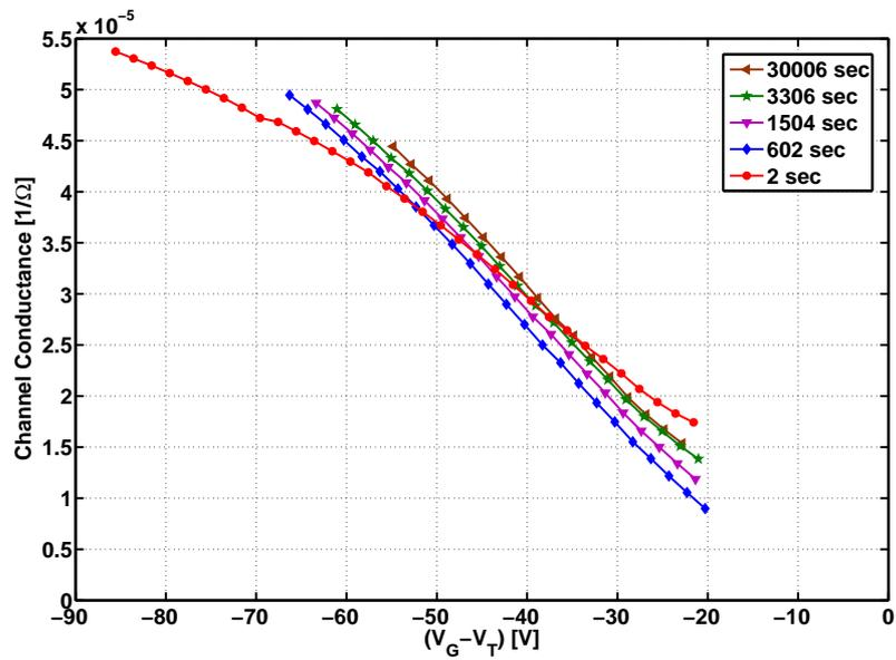
(b) Channel conductance vs. gate voltage minus threshold voltage at different times
