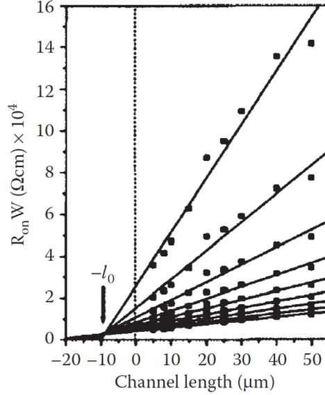
Figure 9.1.: Illustration of the transfer line method. Each line corresponds to a give gate voltage. Picture taken from Ref. [7].
