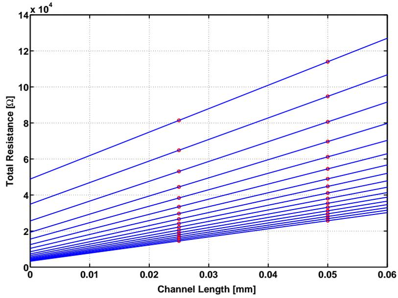
(a) Total Resistance vs channel length for different gate voltage. The extrapolation to zero length gives the contact resistance.
