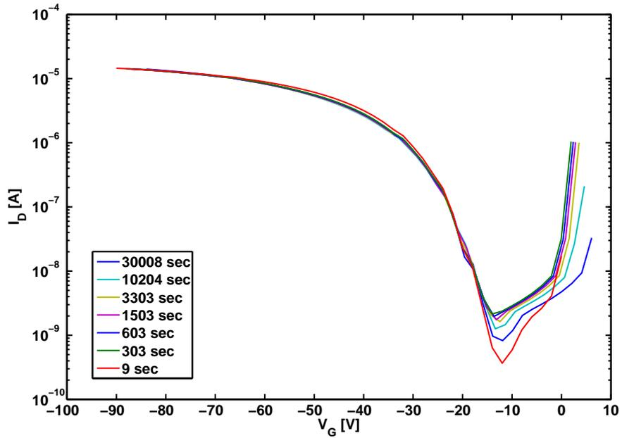
(b) Logarithmic plot of drain current vs.  $(V_G - V_T)$  at different times.
