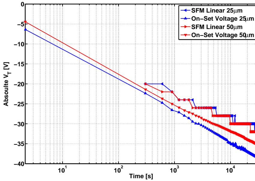
(b) logarithmic plot of absolute threshold shift vs. Time.
