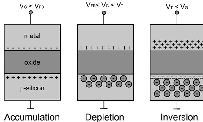
Figure 3.2.: Charges in an Metal-Oxide-Semiconductor structure under accumulation, depletion and inversion conditions. Encircled charges are space-charges.
