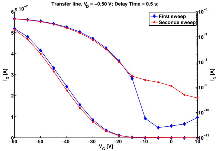
(b) Drain current vs gate voltage. Delay time between each measurement point was 0.5 seconds.
