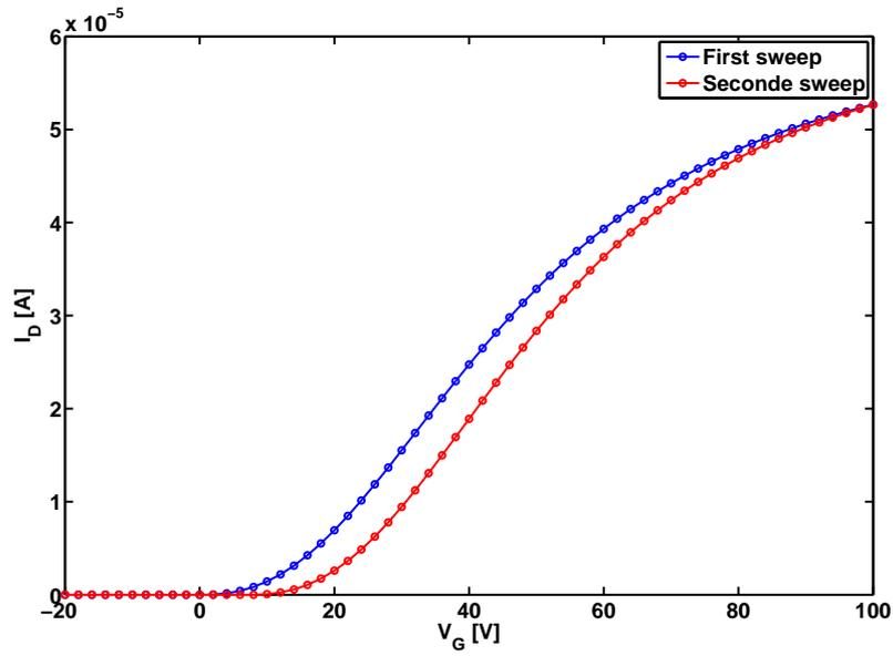
(a) Drain current vs gate voltage.
