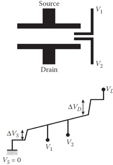
Figure 9.2.: Principle of the four-point probe method. Picture taken from Ref. [7]
