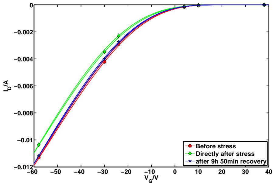
(b) Transfer characteristics at  $V_D = -45V$ . After 10 hours of recovery the transfer characteristic has almost returned to the initial state.
