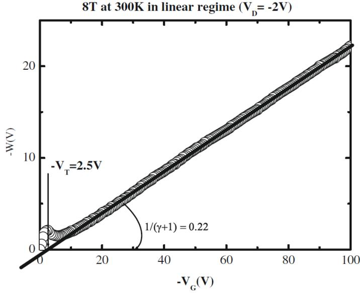
Figure 8.4.: Quantity  $w$  calculated using equation (8.6). For gate voltage higher than  $15V$ ,  $w$  shows linear behavior and can be therefore fitted in this range. Picture take from Ref. [22].
