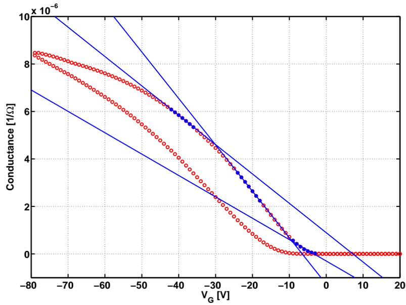
(a) Linear transfer line characteristic at  $V_D = -0.5V$  of a pentacene OTFT. All measurement points in the on-state are located in the linear regime. Fits are performed on three different fitting windows, according to equation 8.1;
