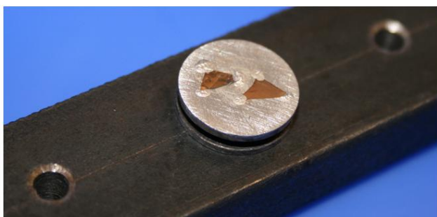
Fig. 4.14. Two triangles of Au coated polycarbonate membrane fixed on a SEM-holder with conductive silver: Triangle on the left side – Au layer on top; triangle on the right side – polycarbonate layer on top
