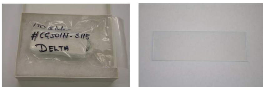
Fig. 4.4. ITO coated glass slides (thickness: 1,096 mm; R_{ITO} = 28 \Omega ) packed (left) and a single one unpacked (right)
