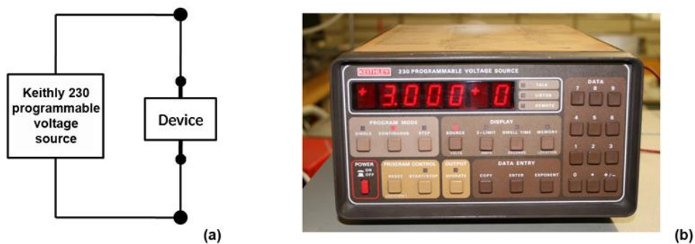
Fig. 6.82. (a)...schematic circuit diagram; (b)...KEITHLEY 230 programmable voltage source
