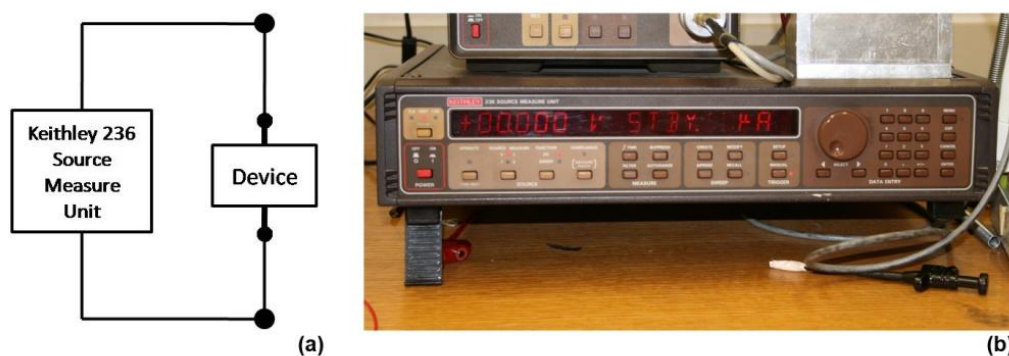
Fig. 5.1. Schematic circuit diagram for cyclovoltammetry (a); KEITHLEY 236 source measure unit (b)
