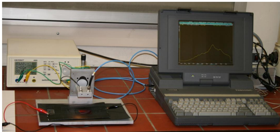
Fig. 5.16. Investigation of the electrochromic devices with the CCD spectrometer during cyclovoltammetry
