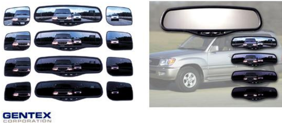
Fig. 3.7. Auto-dimming rearview mirror from GENTEX
