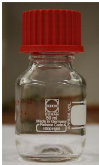
Fig. 6.1. 50 ml gas tight glass vials (DURAN)
