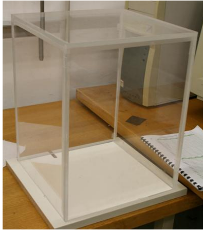
Fig. 6.34. Acrylic plastic cuboid: During the dip coating process the acrylic plastic cuboid was put over the mechanical drawing device to prevent disturbances caused by air circulations
