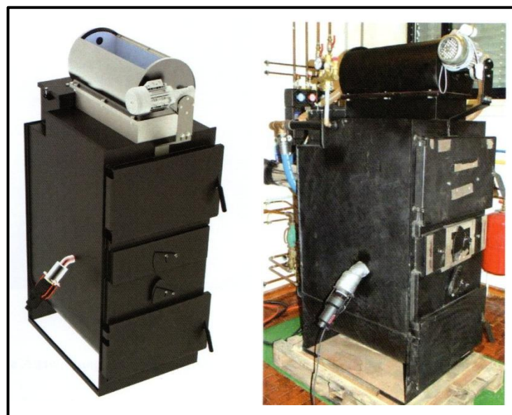
Figure 1-2: Rotary feeder on top of a boiler
