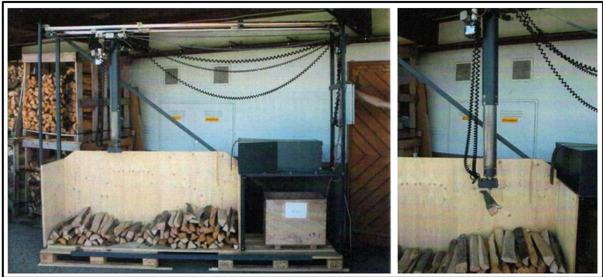
Figure 1-1: Prototype of an automated split log feeding system
