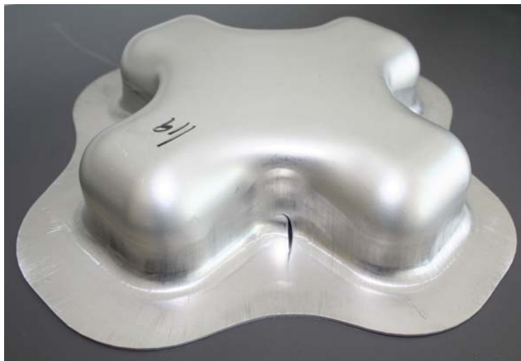
Figure 5-2: Material failure; with thermal treatment
