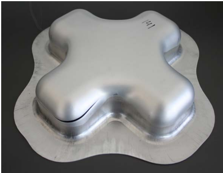
Figure 5-1: Material failure; without thermal treatment
