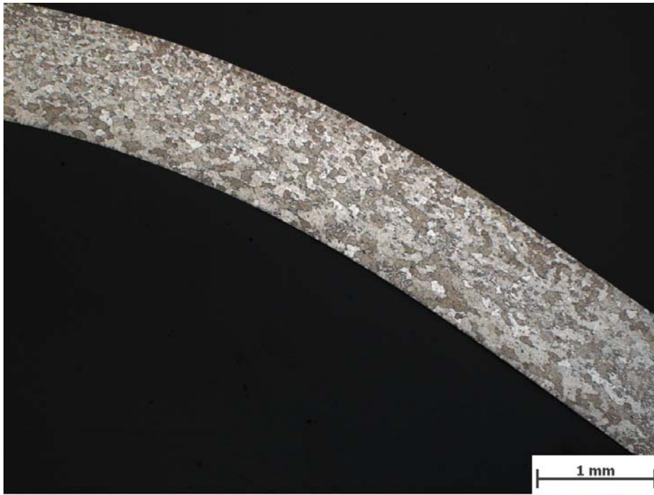
Figure 4-23: Recrystallization Diagram Group 5 – 1311w108
