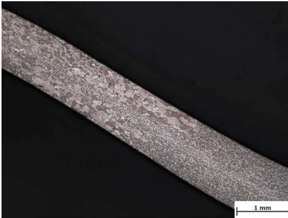
Figure 4-18: Recrystallization Diagram Group 5 – 1311w027
