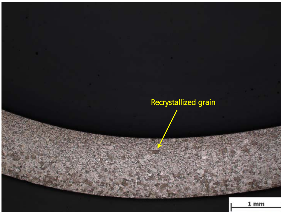
Figure 4-10: Recrystallization Diagram Group 4 – 1311w058
