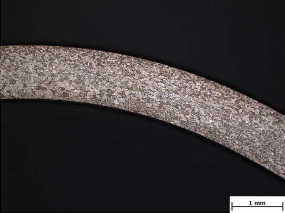
Figure 4-12: Recrystallization Diagram Group 4 – 1311w075
