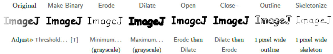
Figure 2.1: A comparison between the different binary operations is presented. This illustration was taken from (Ferreira and Rasband, 2012).
