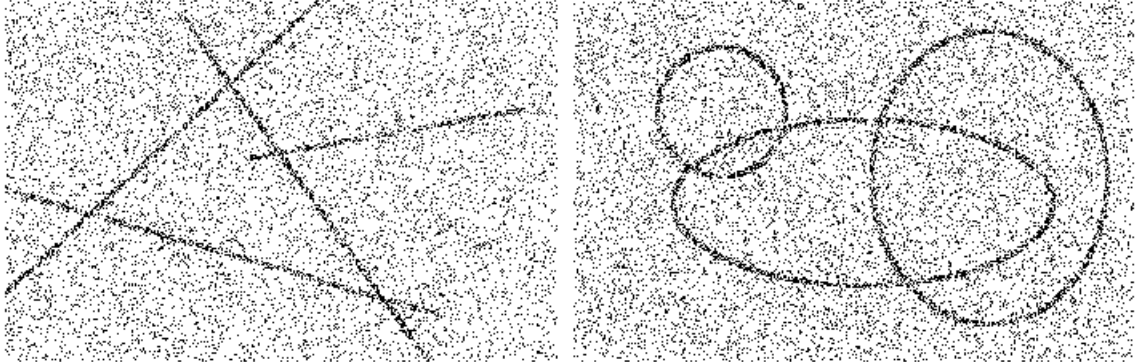
Figure 1.4: For humans it should not be too hard to identify the lines in the left image and the ellipses in the right image and distinguish the structures from the background noise. The task of this sort of feature registration in the field of digital image processing is not so trivial and easy to accomplish. Images were taken from Burger and Burge (2005).
