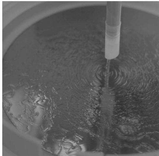
**Figure 3:** Turbulent impinging jet on the rotating disk,  $n = 200 \text{ rpm}$ ,  $Q = 1.2 \text{ lpm}$
