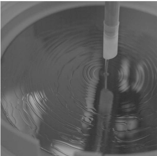
**Figure 2:** Laminar impinging jet on the rotating disk,  $n = 200 \text{ rpm}$ ,  $Q = 0.3 \text{ lpm}$
