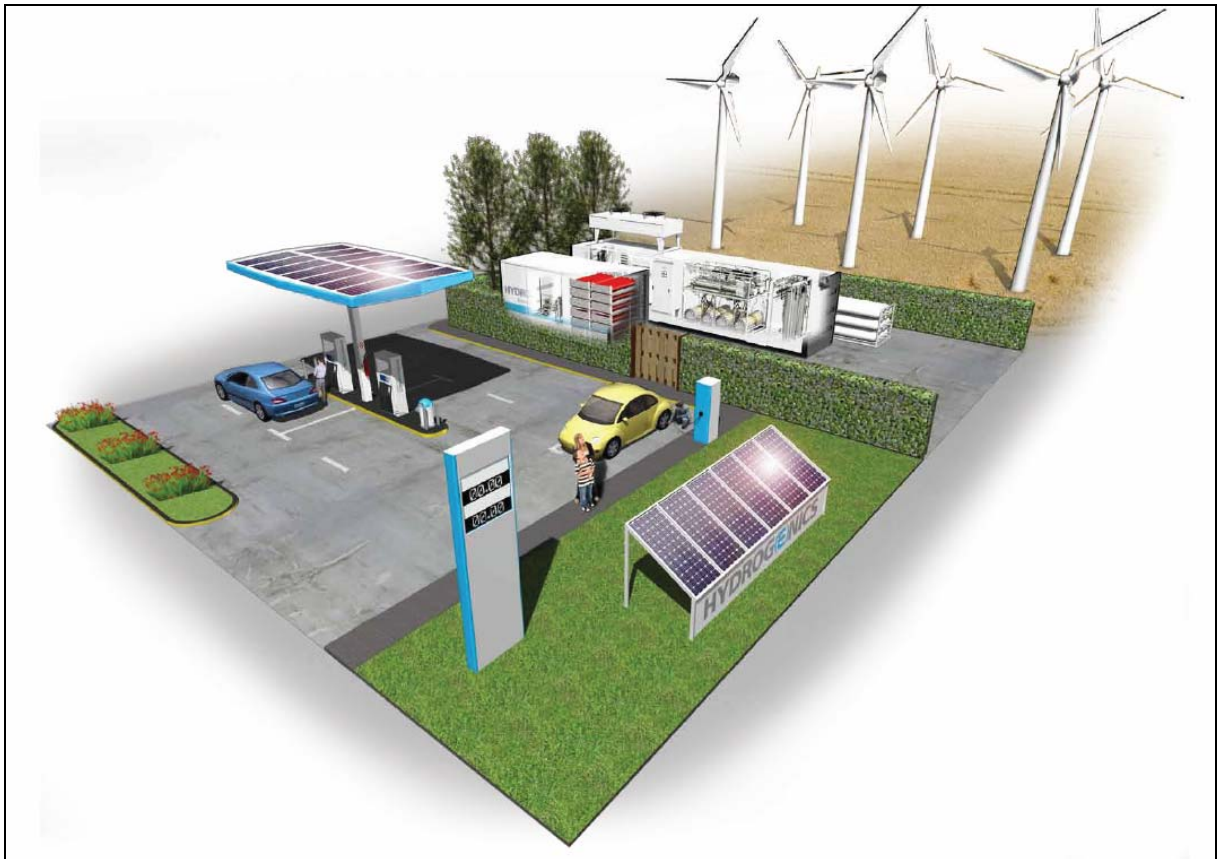
Figure 31: Hydrogenics electrolysis refueling station 39
