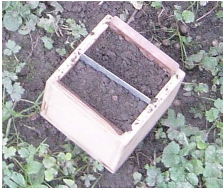
Figure 3.6.: A test device of a dirt-battery with fresh earth
