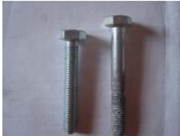
Figure 3.5.: Unused (left) and low-resistive load used (right) zinc-plated screw
