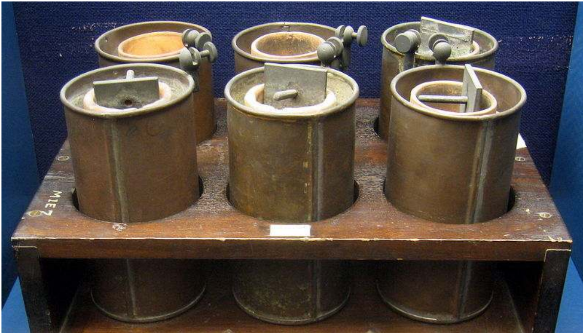
Figure 3.2.: A Daniell Element with six cells [33]
