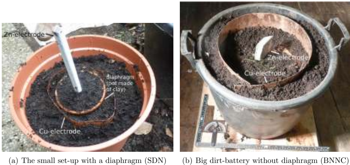
Figure 3.10.: Two different set-ups of dirt-batteries
