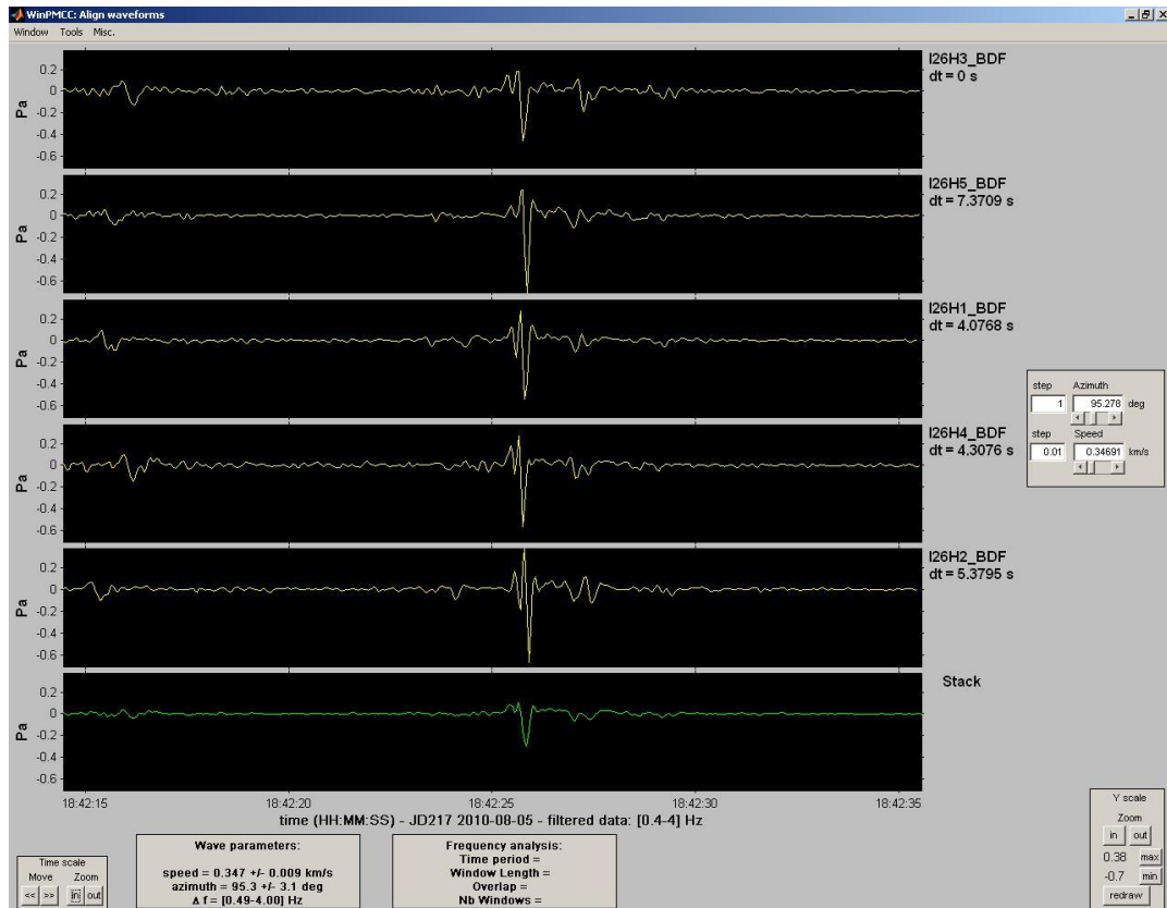
Figure 10-2: Time-aligned signals generated by a single stroke flash
