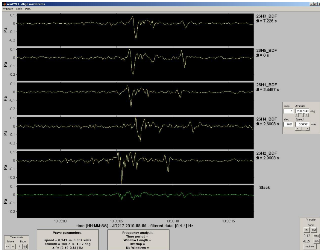
Figure 10-7: Time-aligned signals generated by a flash with two strokes
