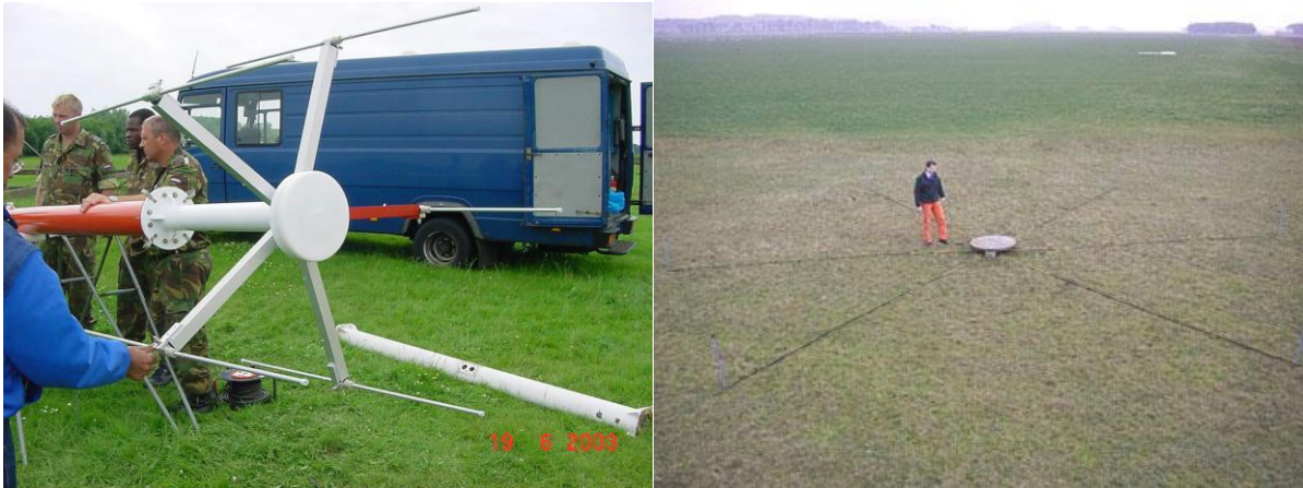
Figure 3-7: The left picture shows the top of a SAFIR station with VHF array and LF sensor. The right picture shows a microbarometer with noise reducer attached constructed of porous hoses. (Holleman, et al., 2006)
