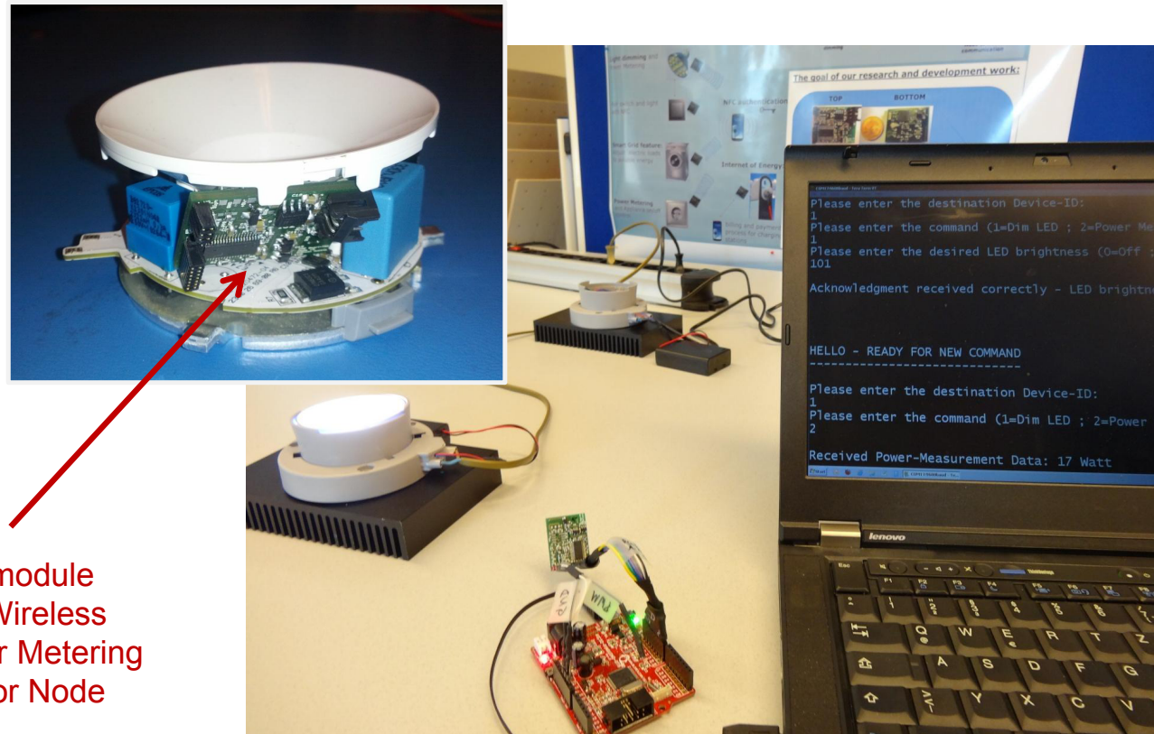
Figure A.6: Power Metering Node integrated into a LED Module, with Power Metering and Dimming Functionality
