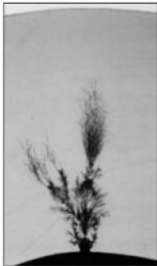
Figure 4.6 Water tree in an PE isolated MV cable [63]
