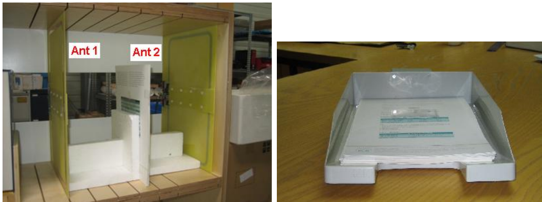
Figure 4.30: Smart shelf and document tray under application conditions
