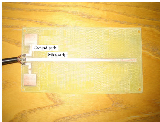
Figure 5.10: Feeding structure of the slot antenna
