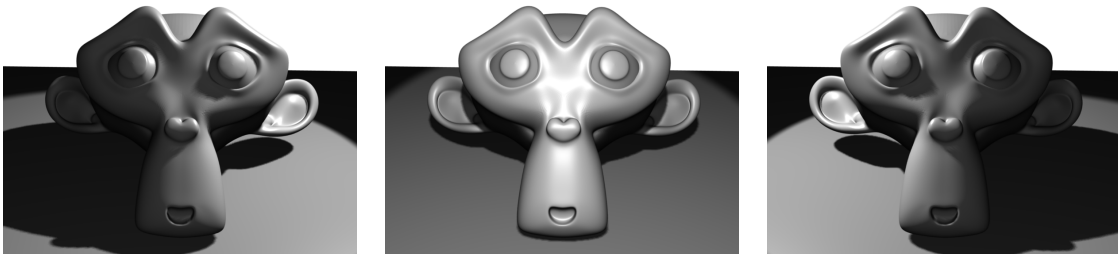
Figure 2.3: Illustration of photometric stereo, which is a technique for estimating surface orientations by observing a scene from the same viewpoint at different illumination conditions.
