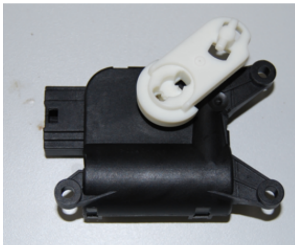
Figure 2.5: Closed HVAC flap control
