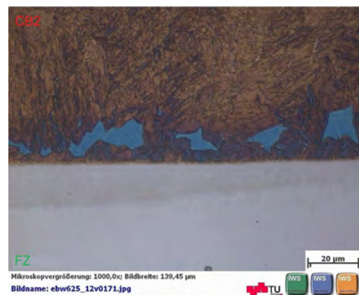
FIGURE 151: DISSIMILAR JOINT, HAZ; D4/11 (4)
