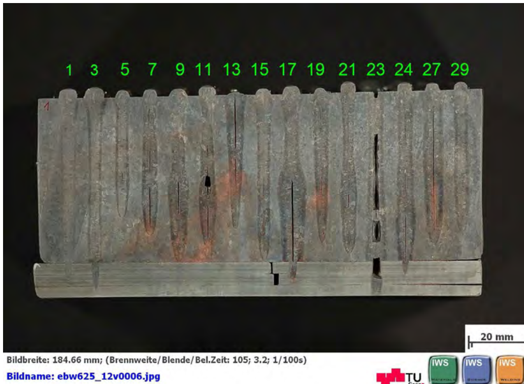
FIGURE 84: CROSS SECTION OF CB2 BLIND WELDING, BLOCK 1
