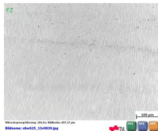
FIGURE 180: MICROSTRUCTURE WPS SPECIMEN, FZ
