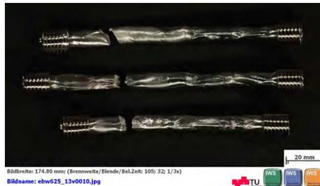
FIGURE 134: TENSILE TEST PIECES, A625 SIMILAR; S3/4
