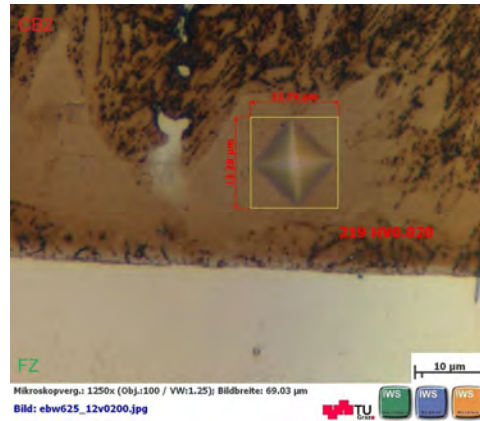
FIGURE 161: MICROHARDNESS DISSIM. JOINT, TEMPERED; D3/23 (2)
