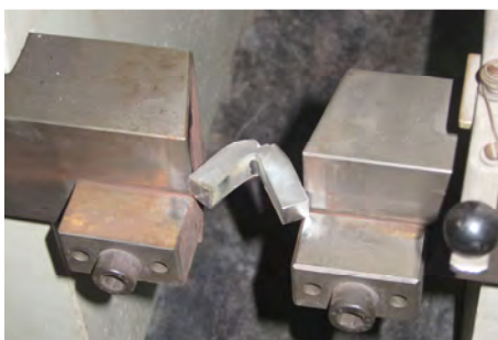
FIGURE 136: STUCK CHARPY TEST SPECIMEN; S7/8
