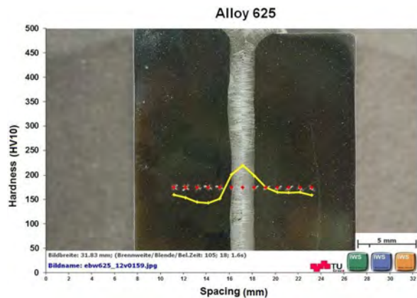
FIGURE 131: HARDNESS LINE HV10, CENTRE; S26/31
