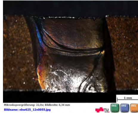
FIGURE 93: #11; CAVITY, MICRO VIEW
