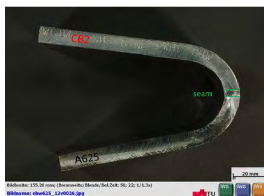
FIGURE 186: SIDE BEND SPECIMEN; SB4
