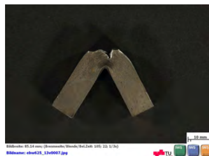
FIGURE 137: CHARPY TEST SPECIMEN; S26/31
