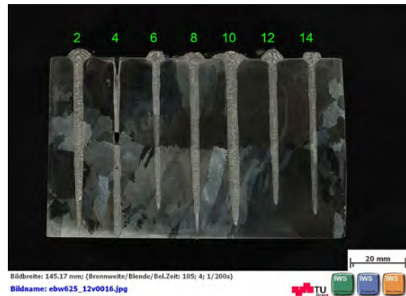
FIGURE 110: BLIND WELDING A625; BLOCK 2
