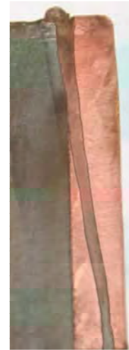
FIGURE 45: BEAM DEFLECTION IN DISSIMILAR WELDING [27]
