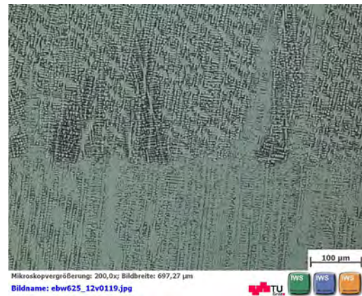
FIGURE 129: CENTRE LINE FUSION ZONE; S3/4 (2)
