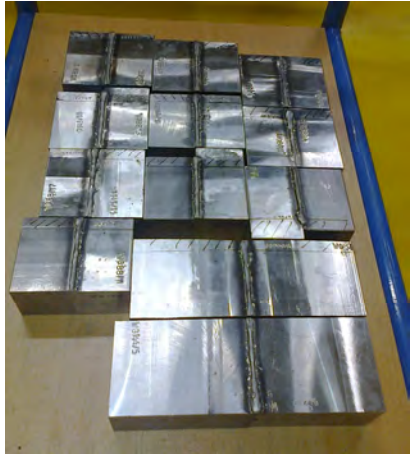
FIGURE 67: SAMPLES FOR MECHANICAL TESTING
