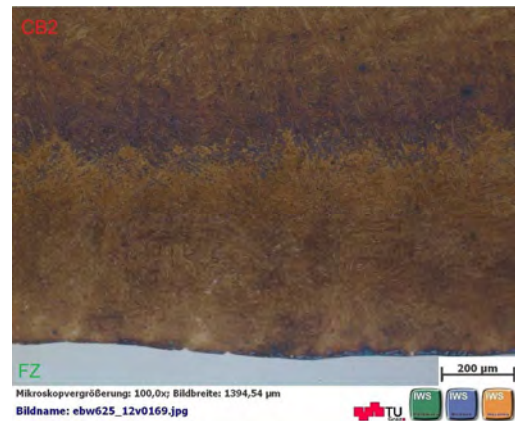
FIGURE 149: DISSIMILAR JOINT, HAZ; D4/11 (2)
