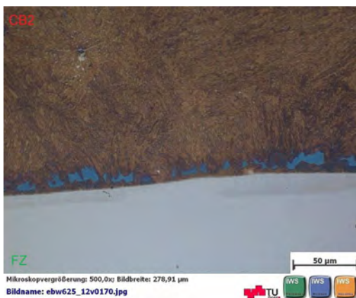
FIGURE 150: DISSIMILAR JOINT, HAZ; D4/11 (3)
