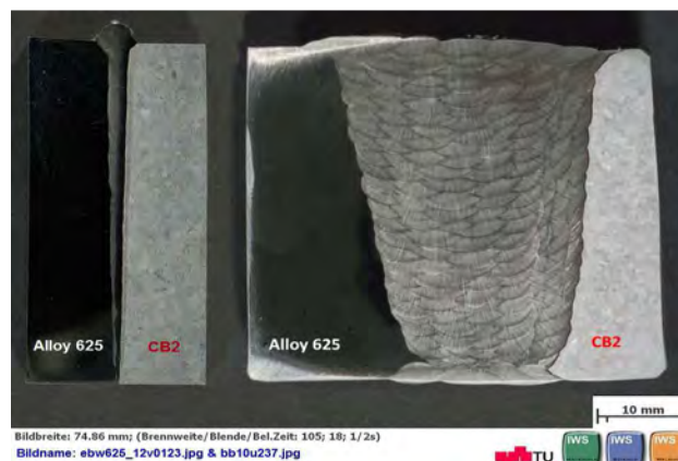
FIGURE 3: COMPARISON EBW TO MAW WITH ROD-ELECTRODE (50MM)
