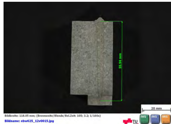
FIGURE 106: BLIND WELDING CB2, BLOCK 4, ETCHED
