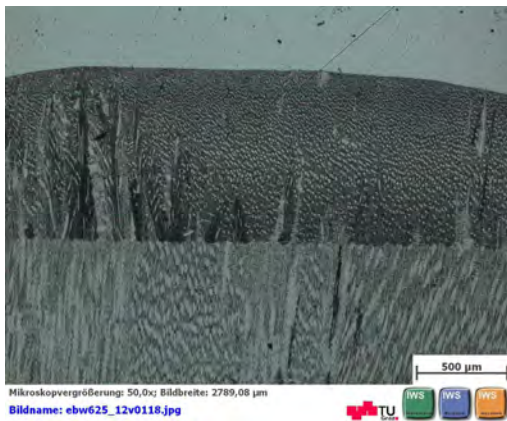
FIGURE 128: CENTRE LINE FUSION ZONE; S3/4 (1)
