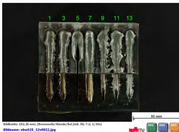
FIGURE 111: BLIND WELDING A625, BLOCK 1, TOP VIEW 1
