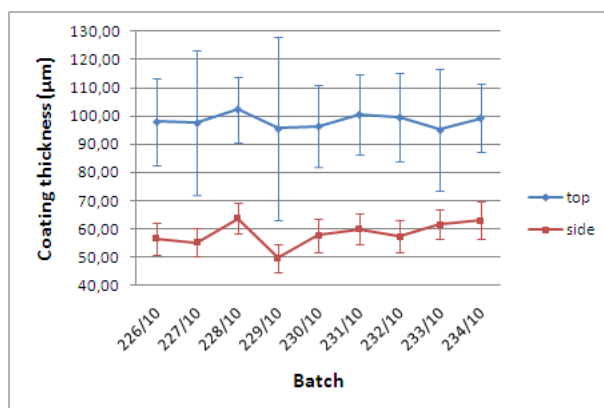
Figure 3.13.: Film coating thickness of tablet B batches, determined with \mu\text{m} -caliper.
