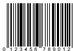
Abbildung 2.2: European Article Number (EAN-13-Barcode)
