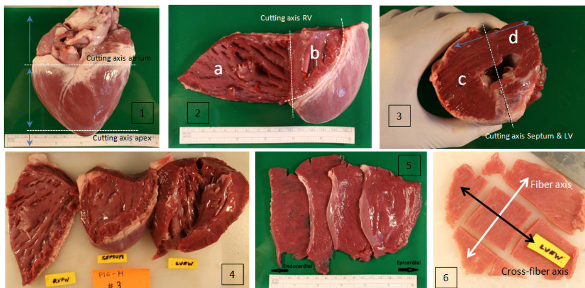
Figure 2.10: This picture shows the different steps of specimen preparation from the PIG Heart #3 for the biaxial tensile tests. The different steps are signed with numbers from one to six. Step 1: cutting axes for apex and atriums; Step 2: cutting of the right ventricles (a) from the septum and left ventricles (b) using the cutting axes; Step 3: cutting axes for separating the left ventricles (c) from the septum (d); Step 4: separated parts of the heart as described; Step 5: extracted tranches from the left ventricles of the PIG Heart #3; Step 6: separating of one specimen for the biaxial tensile test out of one tranche extracted in step 5.
