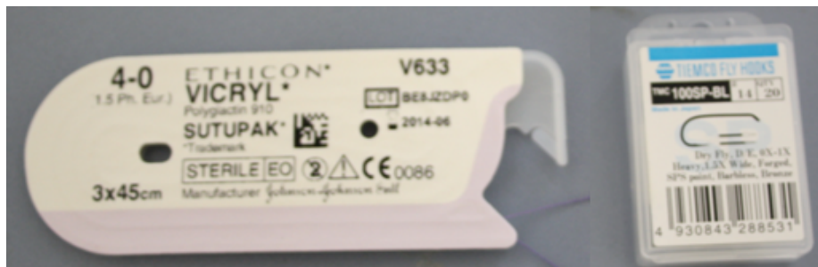
Figure 2.8: Picture of the surgery cords and fishing hooks used for fitting the specimen into the biaxial testing device.
