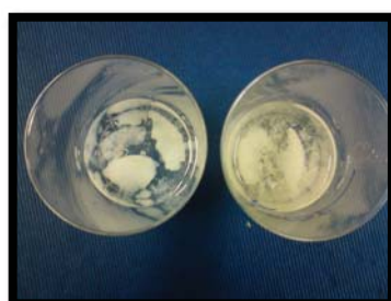
Figure 43 Example of a dextran hydrogel modified upon enzymatic hydrolysis with \alpha -amylase from Bacillus amyloliquefaciens . The blank is on the left and the sample on the right. This image clearly demonstrates the low stability of the dextran hydrogels
