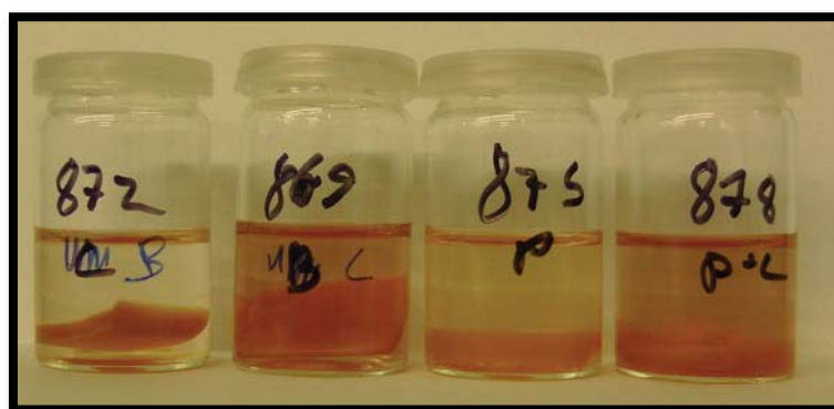
Figure 56 Release of enclosed alizarin from an enzymatically hydrolyzed carboxymethylcellulose hydrogel with pectinase from Aspergillus aculeatus (3U/mL) and cellulase from Aspergillus sp. (4U/mL) B = Blank, C = Samples hydrolyzed with cellulase, P = Samples hydrolyzed with pectinase, CP = samples hydrolyzed with cellulase and pectinase
