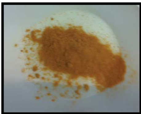
Figure 44 Blend of carboxymethylcellulose and pectin dyed with alizarin
