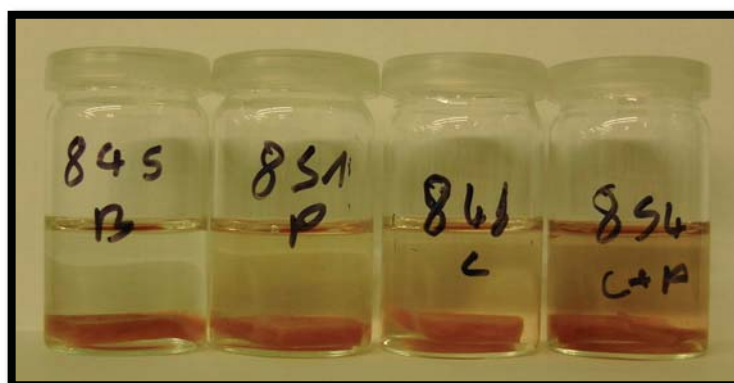
Figure 52 Release of enclosed alizarin from an enzymatically hydrolyzed CMC/pectin (1/1) hydrogel with pectinase from Aspergillus aculeatus (3U/mL) and cellulase from Aspergillus sp. (4U/mL) B = Blank, C = Samples hydrolyzed with cellulase, P = Samples hydrolyzed with pectinase, CP = samples hydrolyzed with cellulase and pectinase
