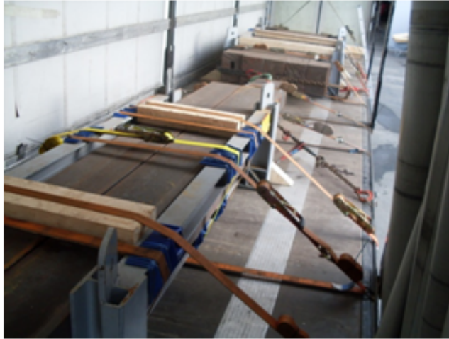
Figure 3: The inside of the trailer with the loaded steel beams
